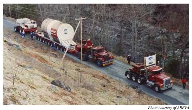
Figure 2-27. Yankee Rowe Reactor Pressure Vessel on Heavy Haul Truck (1997)
