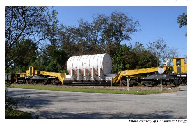
Figure 2-73. Big Rock Point Reactor Pressure Vessel on ETMX1001 Railcar (2003)
