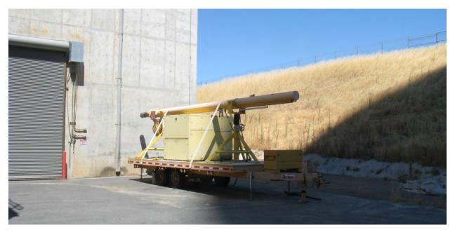
Figure 2-87. Hydraulic Ram Used to Emplace and Withdraw Canisters from Horizontal Storage Modules at Rancho Seco (2013)
