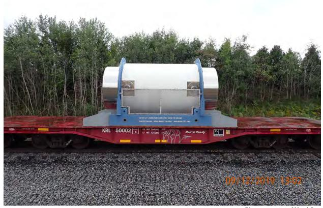
Photo courtesy of NorthStar Figure 2-331. MP197HB Transportation Cask Without Impact Limiters on Railcar (2019)
