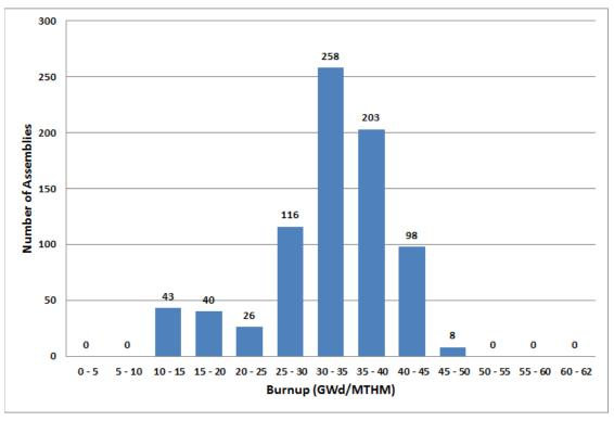
Figure 2-272. San Onofre-2 and San Onofre-3 Number of Assemblies Stored in 24PT4 Canisters versus Burnup (EIA 2013)
