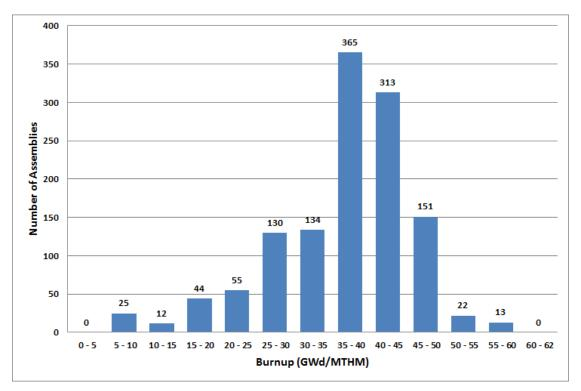
Figure 2-335. Fort Calhoun Number of Assemblies versus Burnup (Data for Assemblies Discharged from 2013 to 2016 Are Preliminary)
