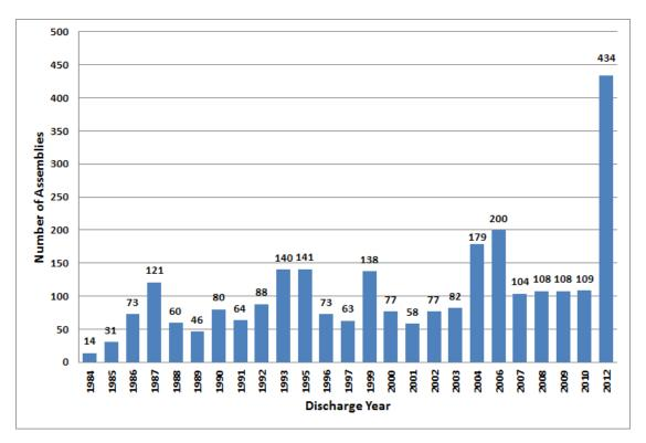
Figure 2-273. San Onofre-2 and San Onofre-3 Number of Assemblies Stored in MPC-37 Canisters versus Discharge Year (EIA 2013)
