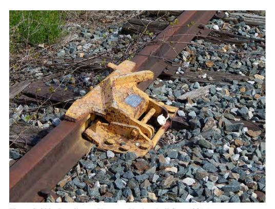
Figure 2-322. Derailer on Vermont Yankee Rail Spur (2016)
