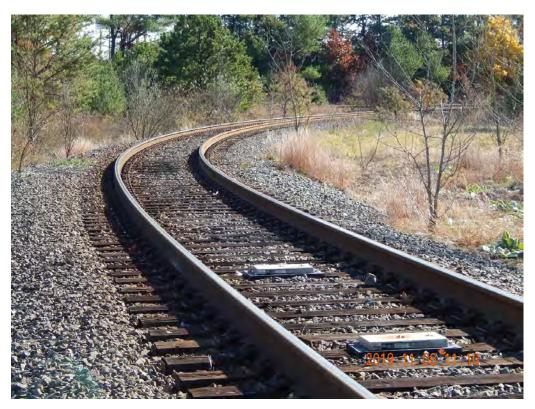
Figure 2-412. Positive Train Control Sensors at First Potential Rail Transload Location (2019)
