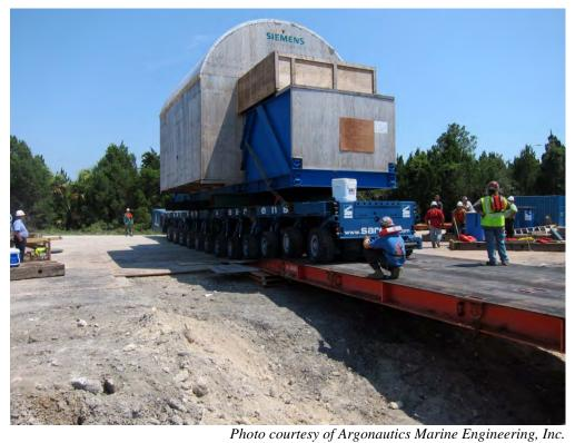
Figure 2-196. Turbine Components Driving Off of Unloading Ramp (2012)
