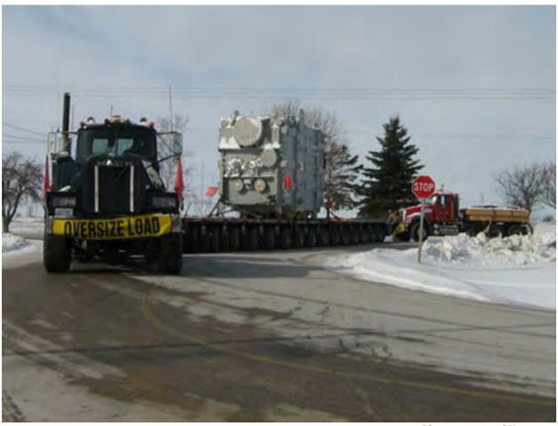
Figure 2-215. Transformer on 15-axle Goldhofer Trailer (2008)
