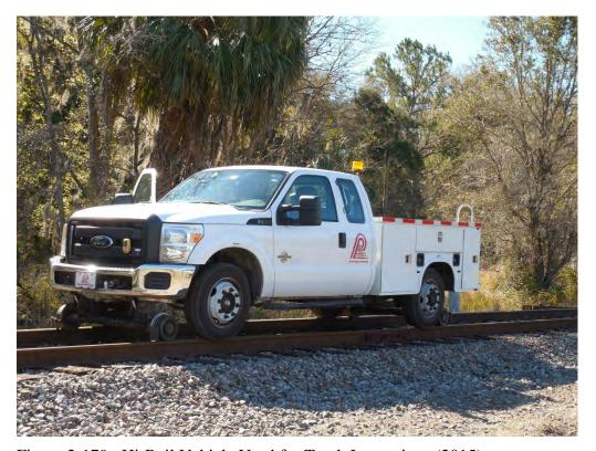
Figure 2-179. Hi-Rail Vehicle Used for Track Inspections (2015)
