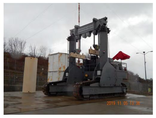
Figure 2-401. Storage System Mover at Pilgrim Independent Spent Fuel Storage Installation (2019)
