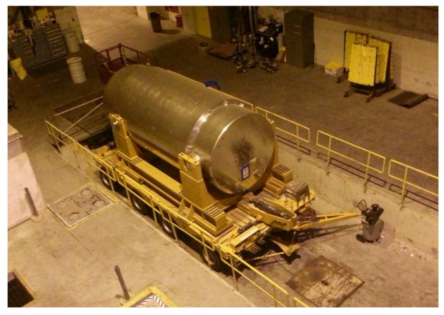
Figure 2-86. MP187 Transportation Cask at Rancho Seco (2013)
