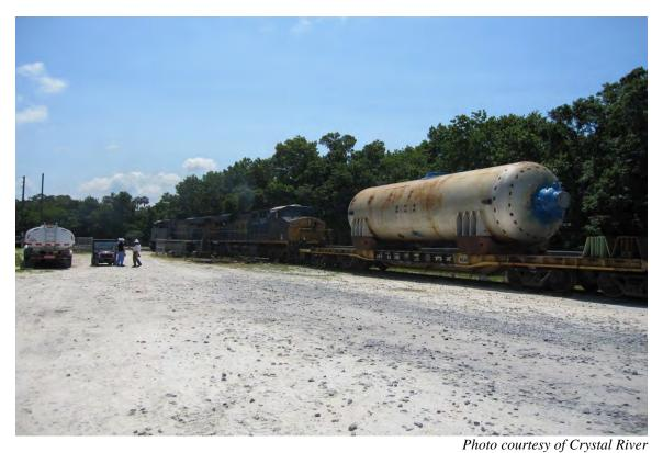
Figure 2-185. Locomotive Picking Up Old Moisture Separator Reheaters (2009)
