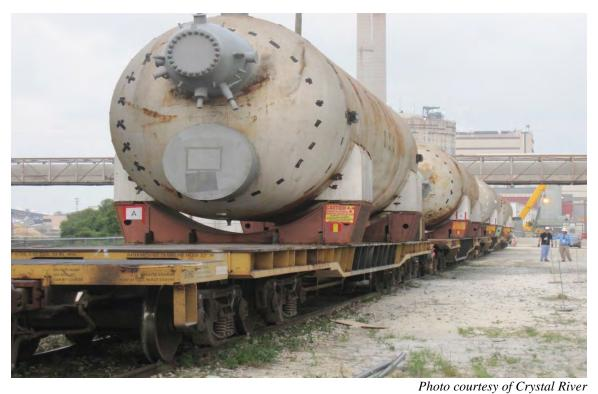
Figure 2-184. Old Moisture Separator Reheaters Being Shipped Off-site by Rail (2009)
