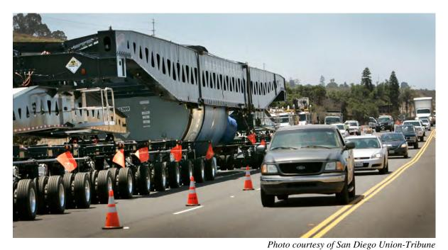
Figure 2-304. Old Steam Generator on Heavy Haul Truck Transporter (2011)
