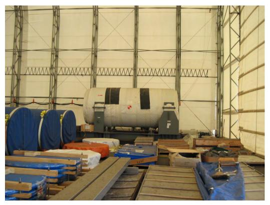
Figure 2-265. Transfer Cask for 32PTH2 Canisters (2015)
