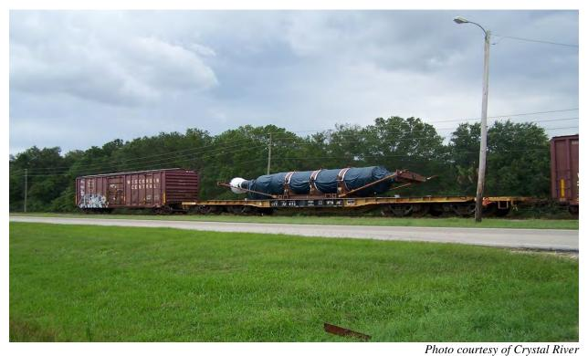
Figure 2-182. Generator Rotor Being Shipped by Rail to the Crystal River Site (2009)
