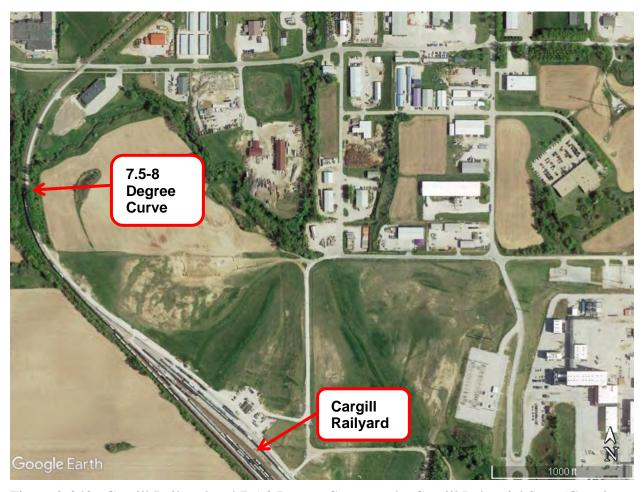
Figure 2-348. Cargill Railyard and 7.5-8 Degree Curve on the Cargill Industrial Spur (Google 2019)
