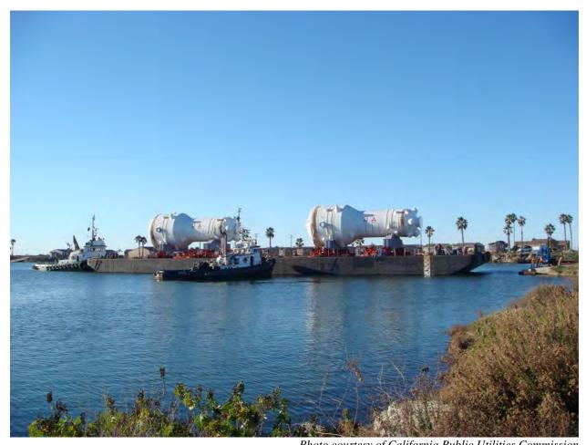
Photo courtesy of California Public Utilities Commission Figure 2-297. San Onofre Steam Generators on Barge Arriving at Del Mar Boat Basin (2009)
