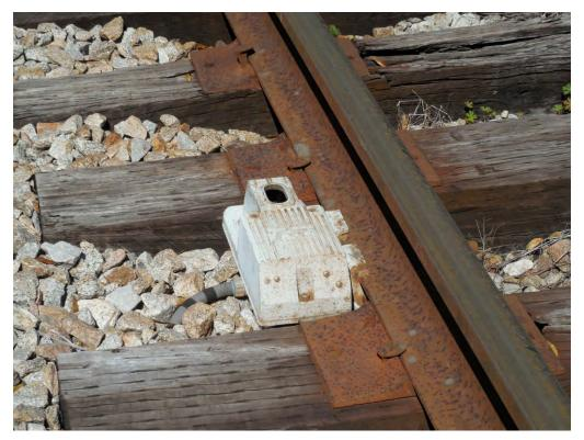
Figure 2-176. Hot Bearing Detector on Florida Northern Railroad (2015)
