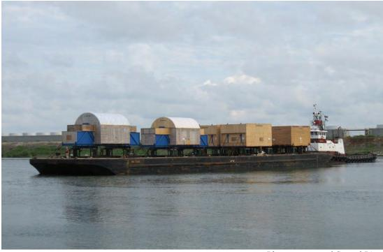
Figure 2-191. Crystal River Turbine Components on Barge (2012)
