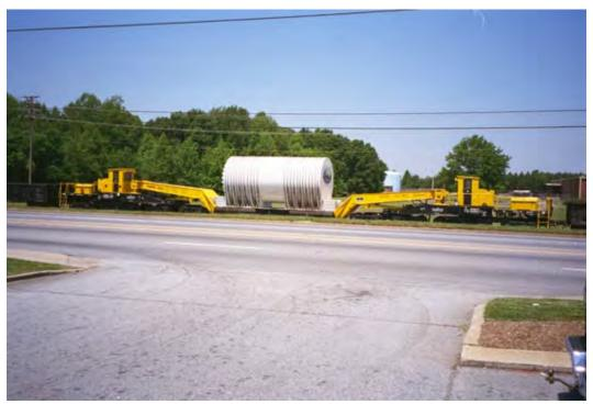
Photo courtesy of Yankee Rowe Figure 2-30. Yankee Rowe Reactor Pressure Vessel on Railcar (1997)
