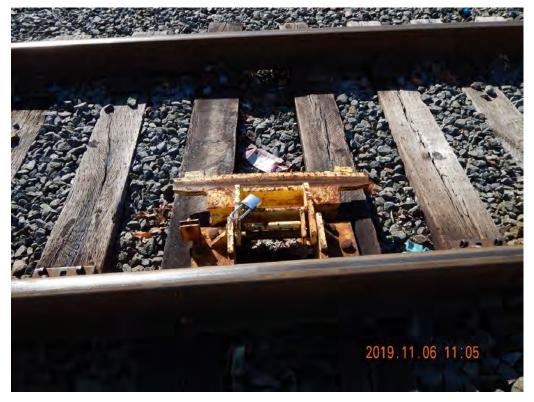
Figure 2-411. Derailer at First Potential Rail Transload Location (2019)
