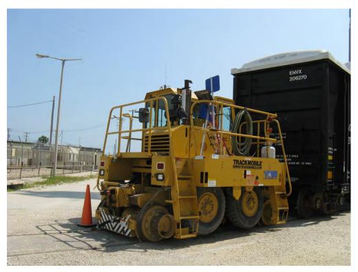
Figure 2-146. Trackmobile Used to Move Railcars On-site (2013)
