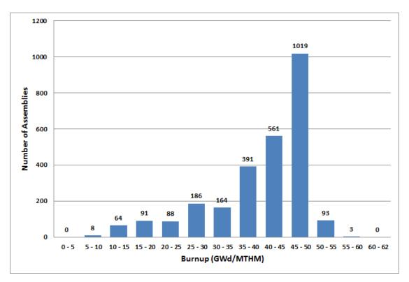
Figure 2-274. San Onofre-2 and San Onofre-3 Number of Assemblies Stored in MPC-37 Canisters versus Burnup (EIA 2013)
