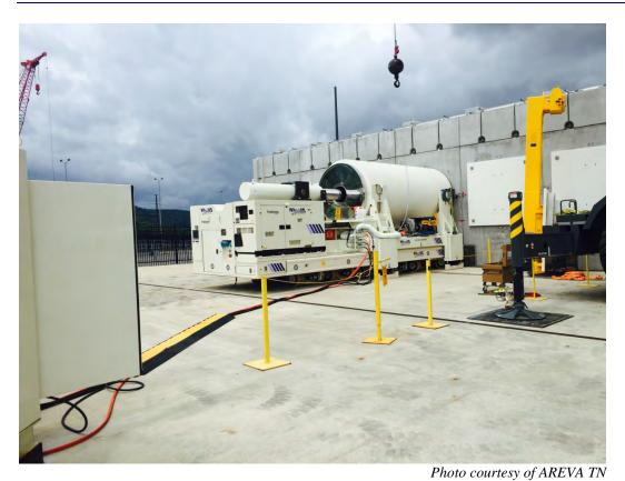
Figure 2-152. Transfer Cask Being Used to Load Canister into Horizontal Storage Module
