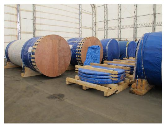
Figure 2-264. 32PTH2 Dry Storage Canisters (On Left) (2015)
