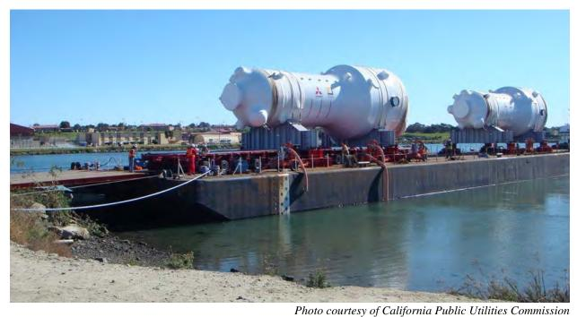
Figure 2-299. Offloading of Steam Generator on Goldhofer Trailer at Del Mar Boat Basin
