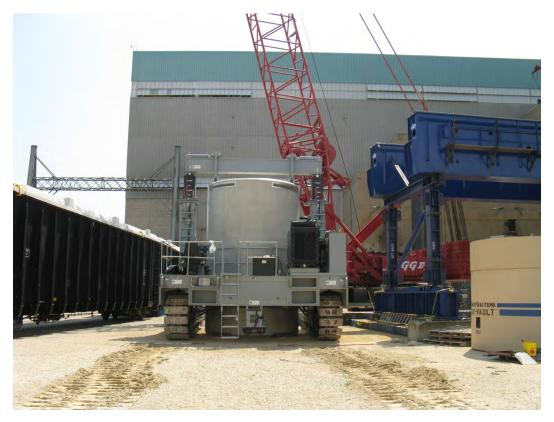
Figure 2-142. Transporter Used to Move Vertical Concrete Storage Casks (2013)
