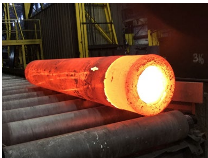
Figure 11. Extruded Alloy 740H AUSC CO 2 steam header pipe. AUSC boilers facilitate collection and sequestration of carbon-base emissions.
