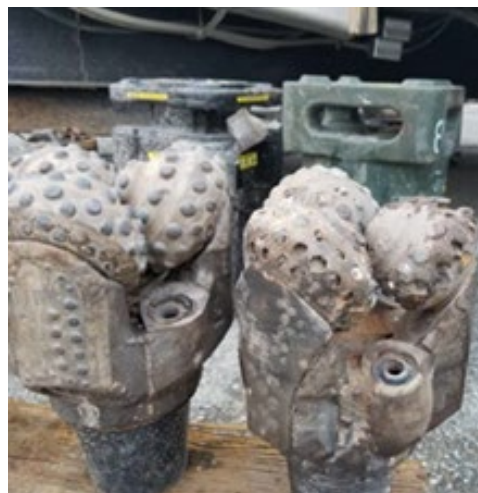
Figure 5. Tricone bits used for geothermal shaft drilling.
