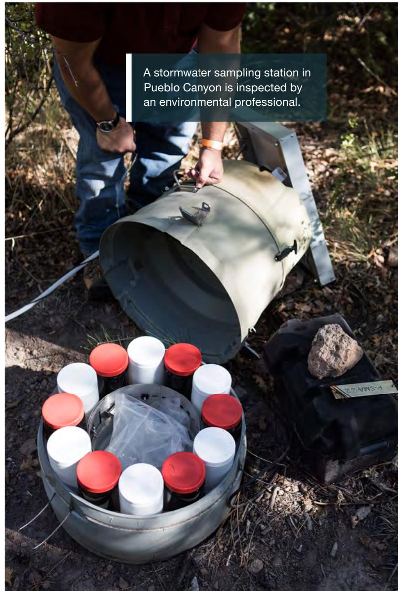
A stormwater sampling station in Pueblo Canyon is inspected by an environmental professional.
