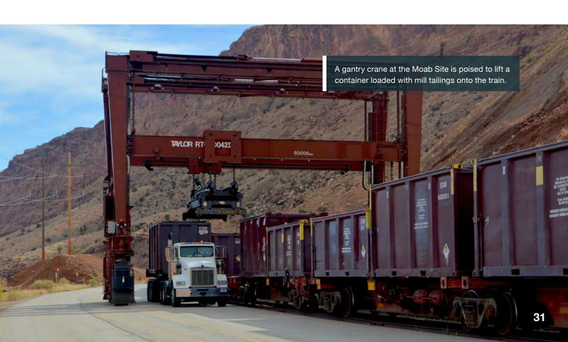
DOE also plans to continue transportation and disposal of oversize debris from the Moab Site, including 14 autoclaves decommissioned by the Atlas Minerals Corporation. They are assumed to weigh at least 40 tons each and could be filled with asbestos. Transportation of oversize debris will continue through CY 2028.
