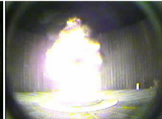
20 MW JP-8 Fire
