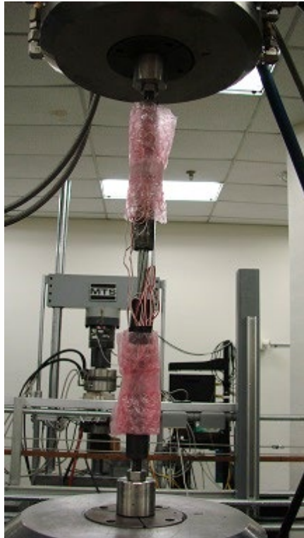
Mechanical testing of connector specimen used to introduce pullout
