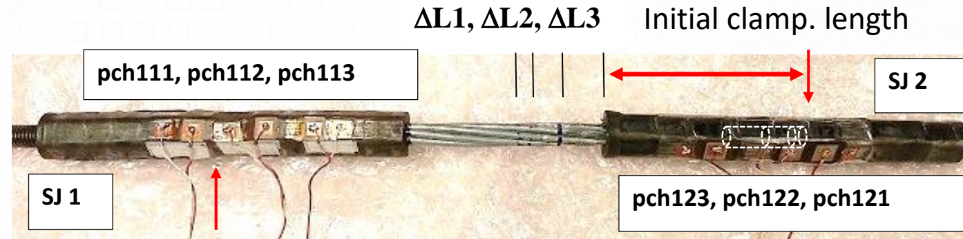
Specimen tested w/ smart patches mounted. Pullouts of steel core \Delta Li ( i = 1, 2, 3 ) are marked.
