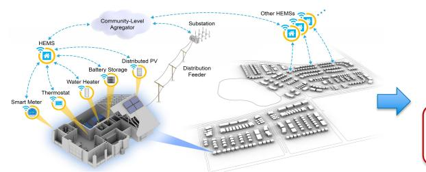
**PV self-consumption** (reduce PV curtailment with flexible loads and batteries)
