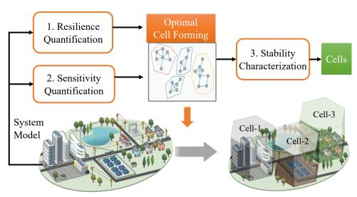
Each identified cell has integrated resilience over a desired threshold and can achieve stable operation when disconnected from the grid.
