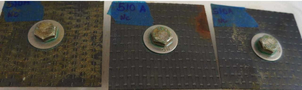
Monel or Ti /CFRP composite fastened samples
