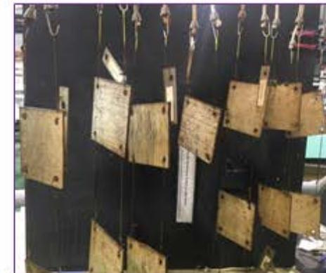
**Corrosion can occur on metals connected to carbon fiber (CF) composites. A special case is crevice corrosion for bolted CF composite immersed in seawater.**
