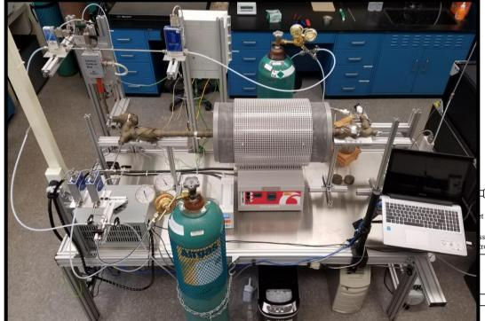
T 293-1873 K  $p_{\text{tot}}$  0.2 mbar-1.01325 bar  $f(T, p H_2, p H_2O)$
