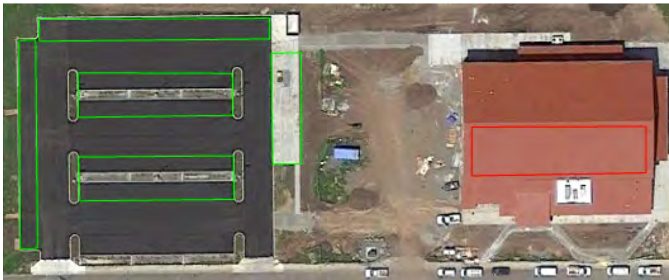
Figure 4: Recreation Center Carport and Rooftop PV System
