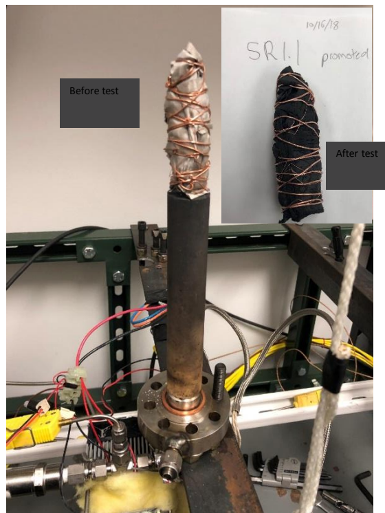
Samples are individually wrapped in steel mesh and bound with copper wire, after test the mesh is substantially oxidized
