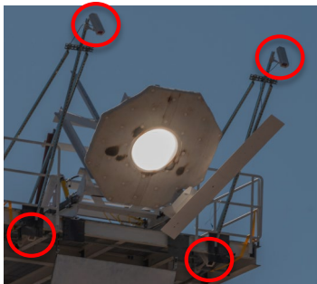
Computer vision based closed-loop tracking: System for Observing Heliostat Orientations while Tracking (SOHOT)
