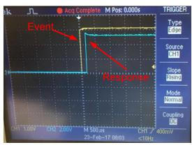
End-to-end delay time for the embedded sequence hopping implementation is **250 micro seconds**
