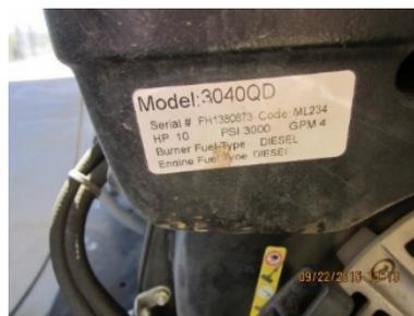
Figure 37. Pressure washer rating and manufacturer's information
