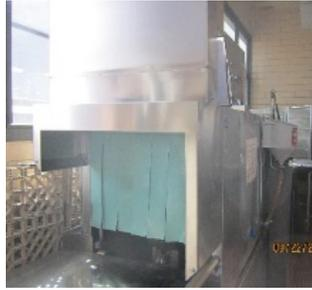
Figure 23. Conveyor-type dishwasher
