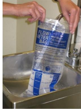
Figure 2. Metered flow bag
