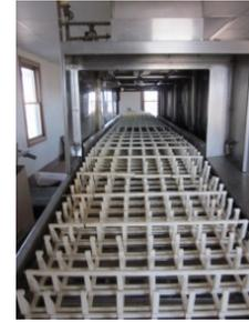
Figure 24. Flight-type dishwasher
