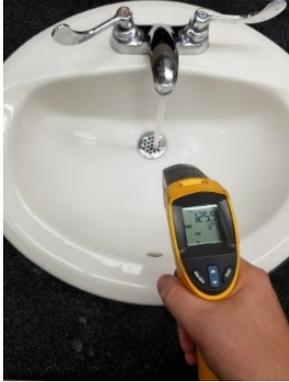
Figure 1. Infrared temperature sensor/gauge
