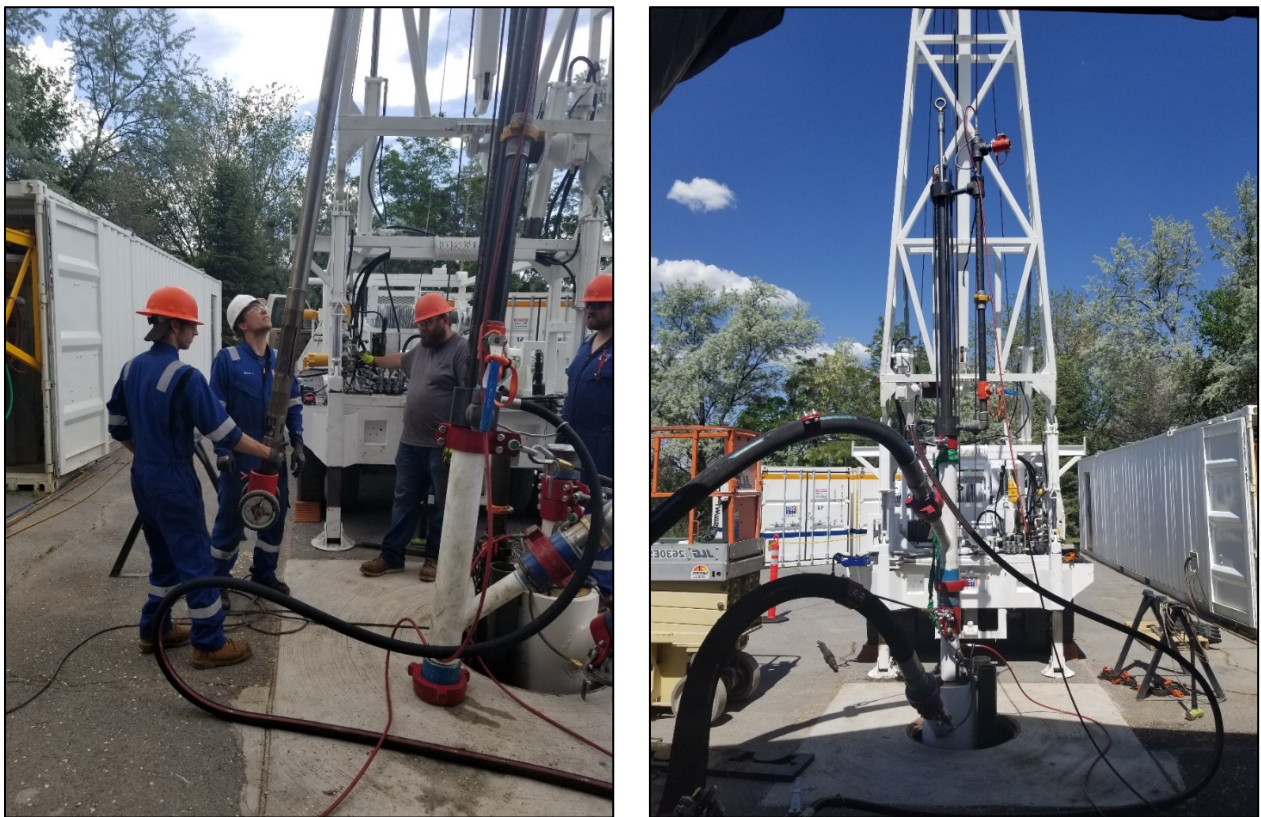
Figure 5: Pressure coring tool bench testing operations conducted by UTA and Geotek in preparation for ultimate deployment during Gulf of Mexico Expedition GOM2-2.
