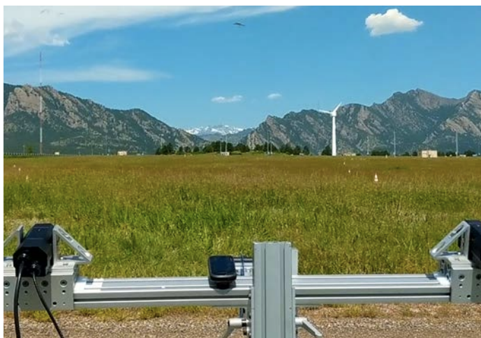
ThermalTracker-3D tracks an unmanned aerial system (visible top, center) during testing at the NREL's Flatirons Campus. Photo by Shari Matzner, PNNL
