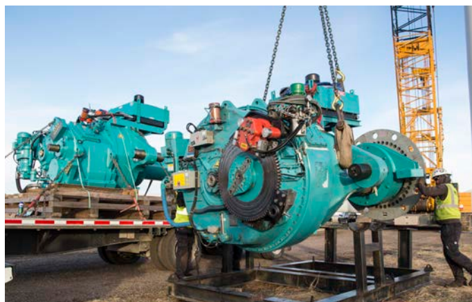
To gather data on the true operating conditions of the turbine's drivetrain, NREL researchers replaced an existing gearbox (front) with a fully instrumented Winergy gearbox and SKF main bearing in the DOE-owned GE 1.5-megawatt wind turbine at NREL's Flatirons Campus. Photo by Dennis Schroeder, NREL
