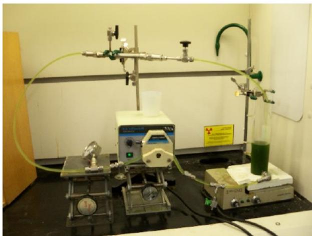
Recirculating Membrane Test System
