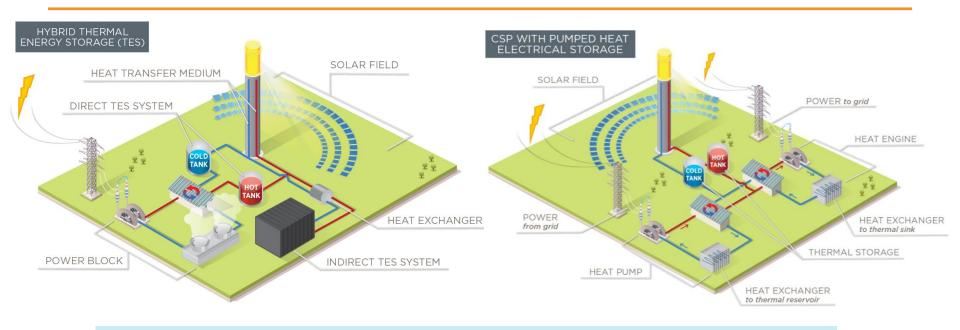
Existing power block at a CSP plant can be leveraged for high value 'indirect' TES:
