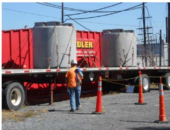
**Figure 2-5. IP-2 Transportation Package Used at SPRU**
