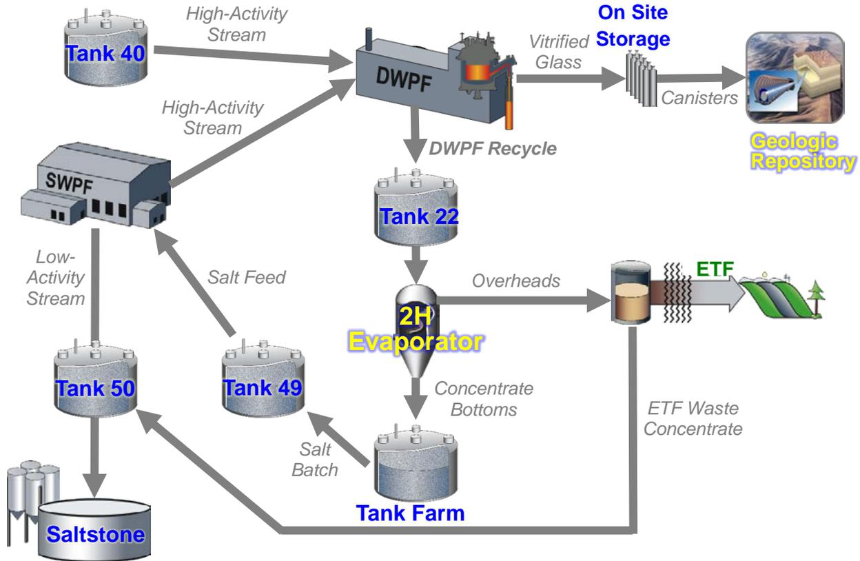
**Figure 2-1. Current Process Flow for DWPF Recycle Wastewater**
