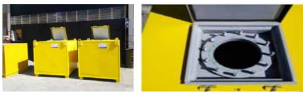
Figure 2. Example of packaging used to transport liquid LLW (side and top view).
