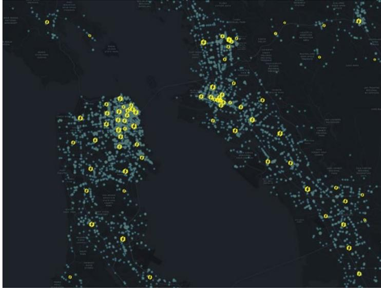
**Figure 17. BEAM-simulated PEV Public Charging Demand from Unconstrained Network (Background) and EVI-Pro Synthesized Charging Station Locations.**
