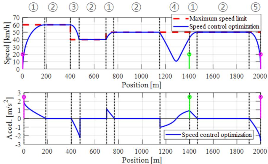
Figure 3-84. Speed (top) and acceleration (bottom) trajectory of speed control optimization for a simple scenario where there are two stops (vertical magenta lines) and one traffic signal (vertical green line). Red dotted line is the varying maximum speed limit.
