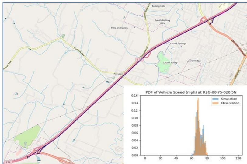
**Figure 3-122. Corridor modeled in VISSIM and histogram of observed vs simulated vehicle speeds in the 20.5 N mile marker.**
