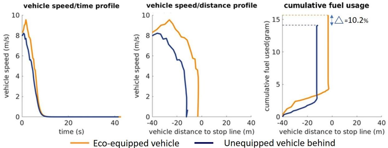
Figure 3-23. EAD Scenario 2: An unequipped vehicle follows an eco-equipped vehicle.
