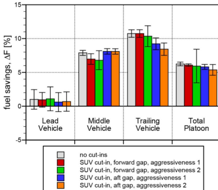
Figure 3-3. Impact of SUV cut-in/out for three vehicle platoons and controller-reaction scenarios (105 km/h target vehicle speed, 29,500 kg vehicle mass).
