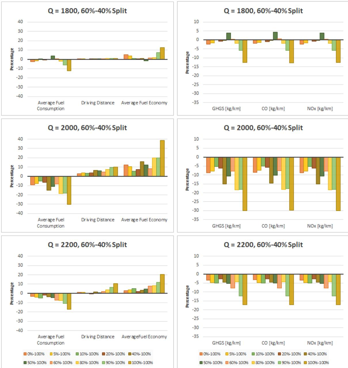
Figure 3-110. Average fuel consumption, driving distance, fuel economy, and emissions changes compared to baseline over the 1 km corridor for three traffic demands (1,800 veh/h, 2,000 veh/h, and 2,200 veh/h; 60%–40% split between the main and ramp roads) with various CAV market penetration rates (numbers in the legend identify the percentages of light- and heavy-duty CAVs).
