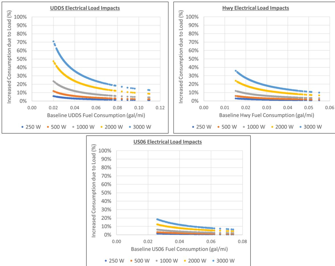
Figure 3-33. MY2019 ICE estimate electrical load sensitivity for UDDS, HWFET, and US06 cycles.
