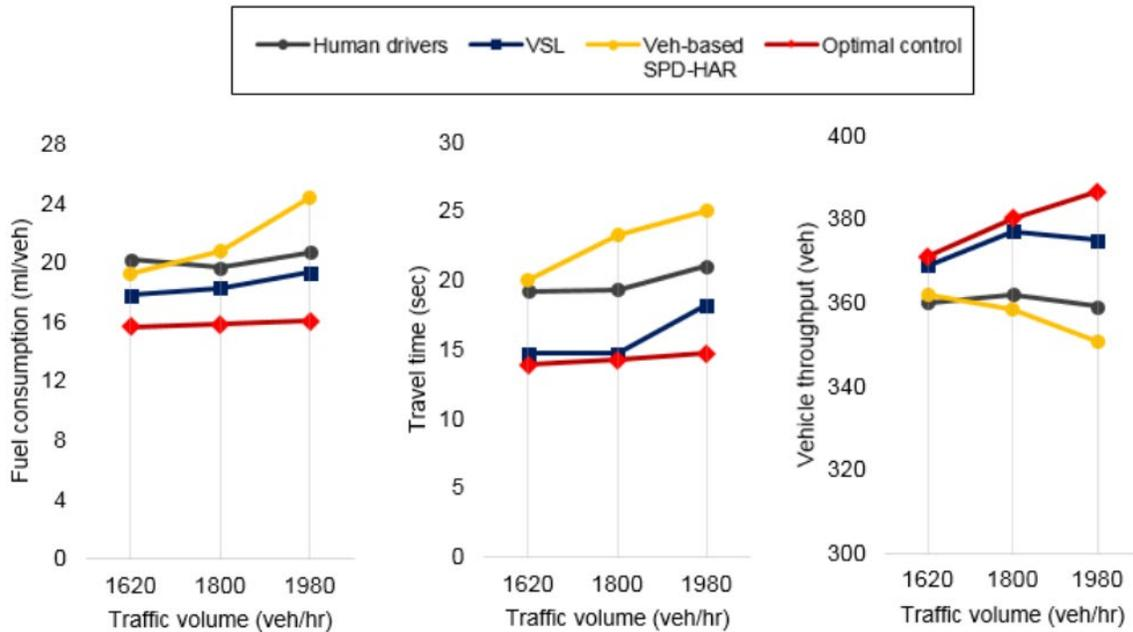
Figure 3-106. Comparisons of the baseline scenario (human-driven vehicles), VSL, and optimal control algorithm.
