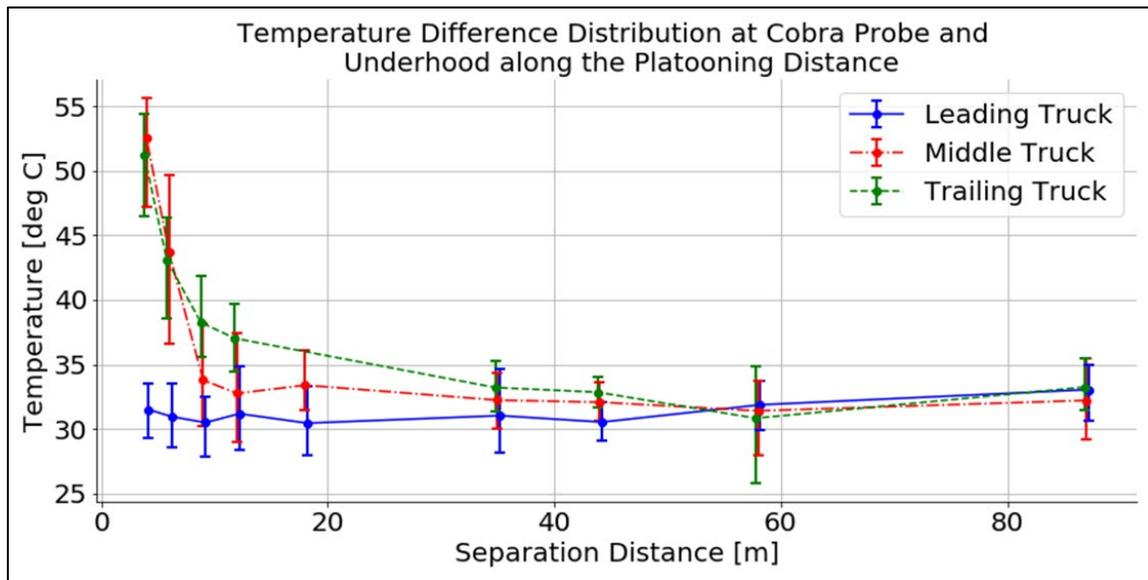
Figure 3-8. Temperature difference at varying separation distances.
