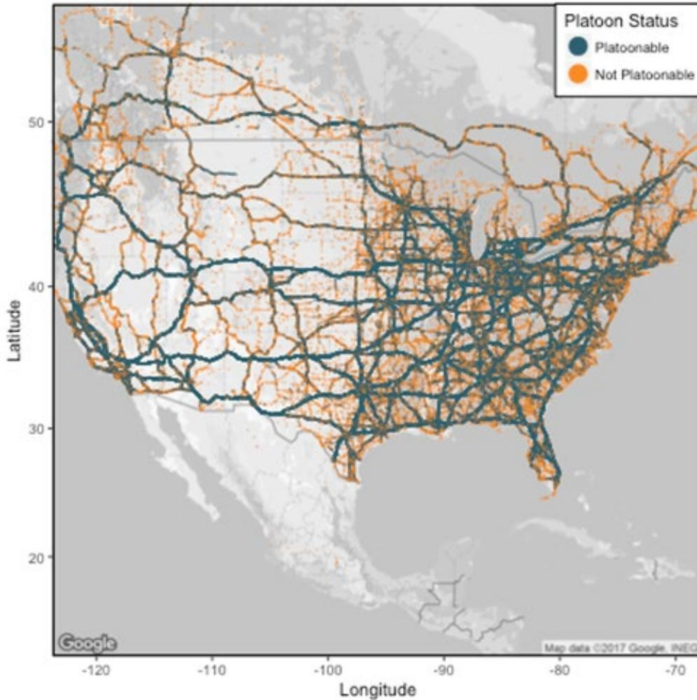
**Figure 3-11. Snapshot of U.S. platoonability based on partner analysis for a single day. Observations with speeds less than 30 mph are omitted for clarity.**
