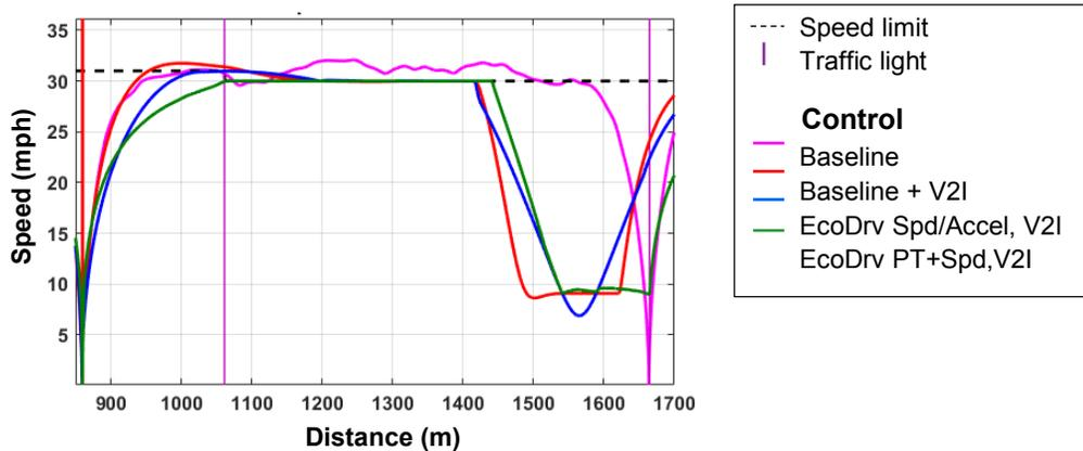
Figure 3-90. Speed traces for a BEV with different control strategies on a short segment with traffic light at 1,670 m.
