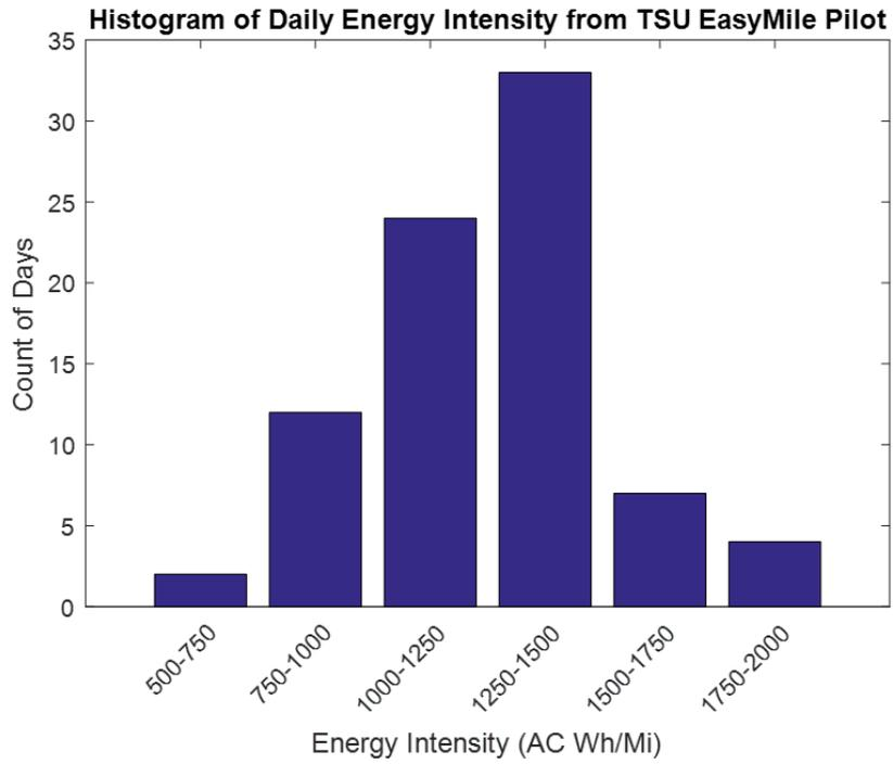
Figure 3-49. Distribution of TSU EasyMile shuttle energy intensity.
