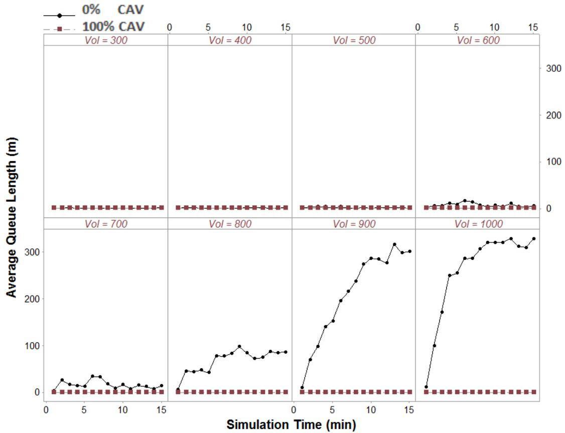
Figure 3-113. Average queue length for eastbound traffic, volume given in veh/h.
