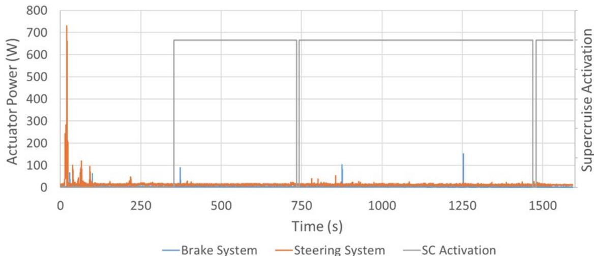
**Figure 3-39. Example Cadillac CT6 braking and steering actuator loads during operation.**
