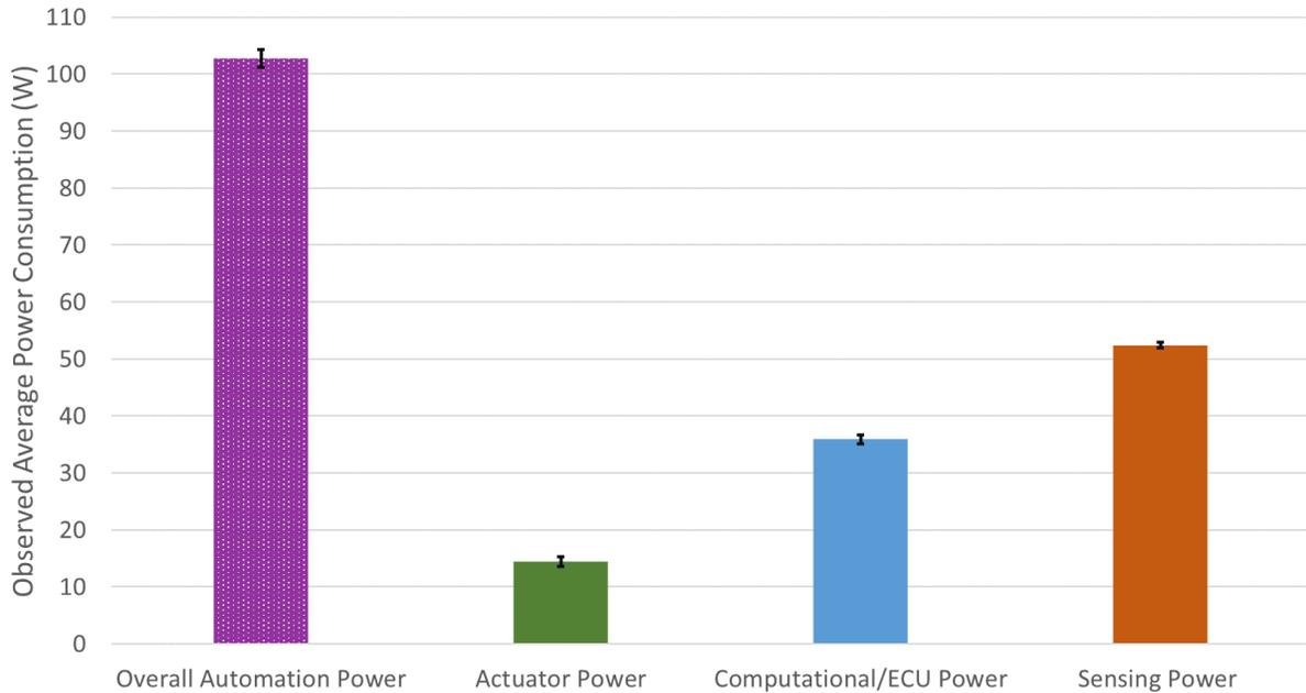
Figure 3-38: Super Cruise overall automation system and subsystem average electrical loads during operation on public limited access highways (95% confidence interval shown in error bars).
