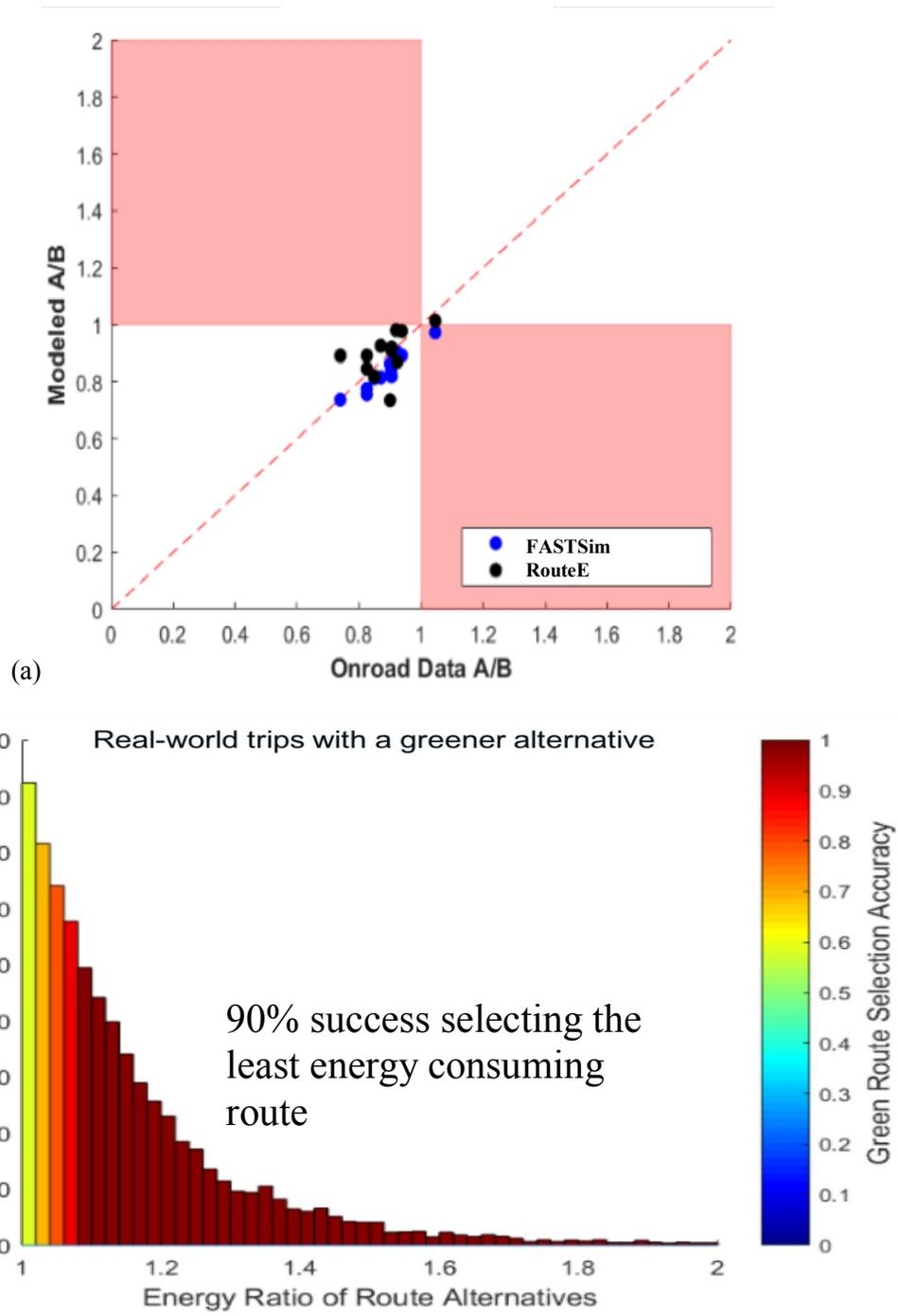
Figure 3-28. Green routing methodology assessment - (a) The plot highlights regions that indicate correct (white) and incorrect (red) selection of the least energy-consuming route option by the basic FASTSim (blue) and RouteE (black) models and (b) estimated success rate identifying the greenest route based on the RMSE from on-road validation of the RouteE model. The distribution demonstrates that the model will accurately select the least energy-consuming route for 90% of real-world trips.
