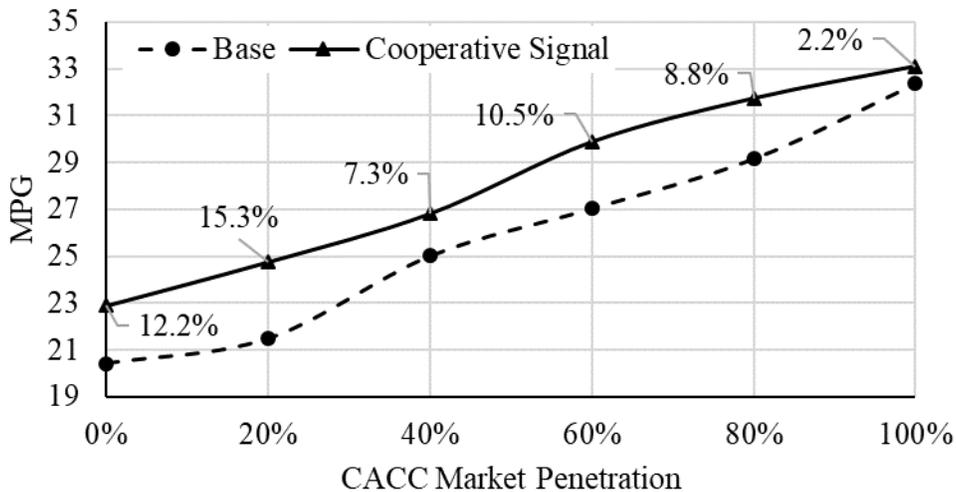
**Figure 3-103. Average vehicle fuel economy (MPG) at an urban signalized intersection under various CACC market penetrations with and without cooperative signal controller.**
