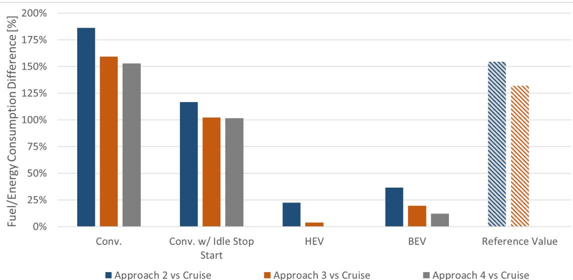
**Figure 3-18. Summary of the fuel and energy consumption of approach strategies 2 through 4 for Scenario 2 compared to cruising (approach 1) through the intersection without stopping for Scenario 2 (patterning denotes reference values).**
