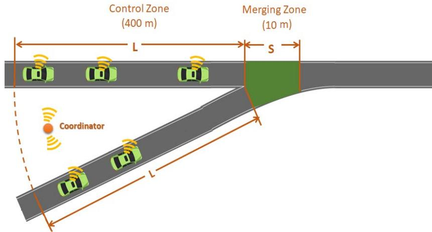
Figure 3-107. Simulated merging on-ramp.
