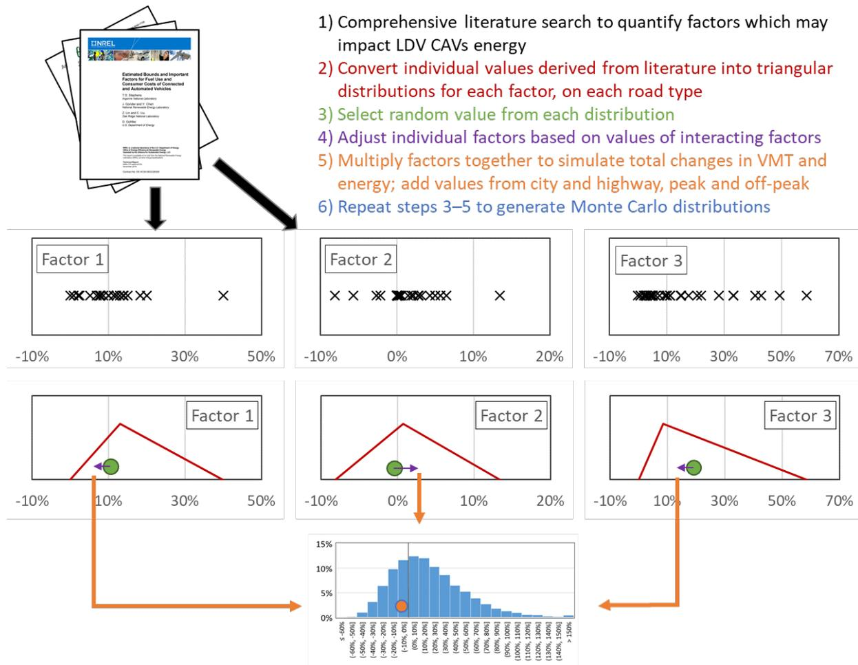
Figure 2-2. Analytical framework for CAVs Synthesis Study.
