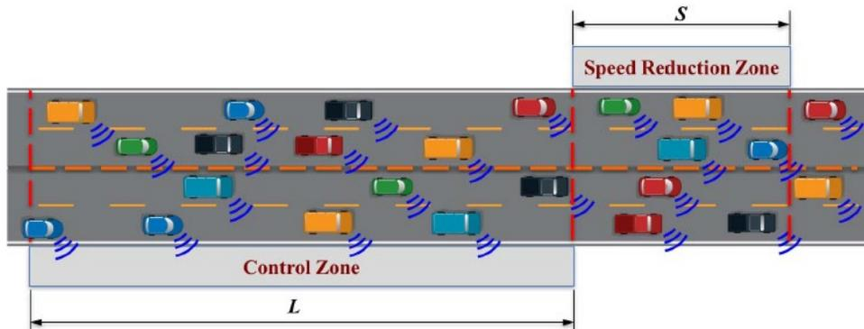
Figure 3-104. Automated vehicles within a control zone approaching a speed reduction zone.
