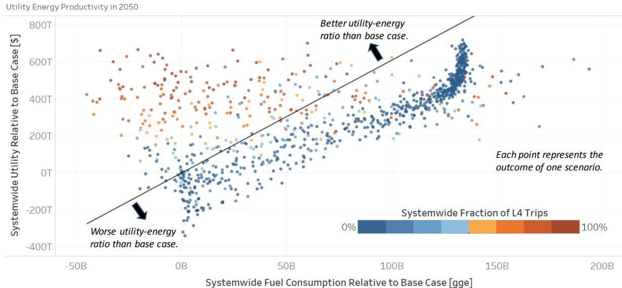
**Figure 3-73. Outcomes (for the comprehensive study) with higher “traveler satisfaction” (system-wide utility) tended to require more fuel consumption unless CAVs Level 4 travel concepts predominate. System-wide utilities showed a linear relationship to fuel consumption in low L4 CAV adoption scenarios, but that did not persist at high L4 CAV adoption levels.**
