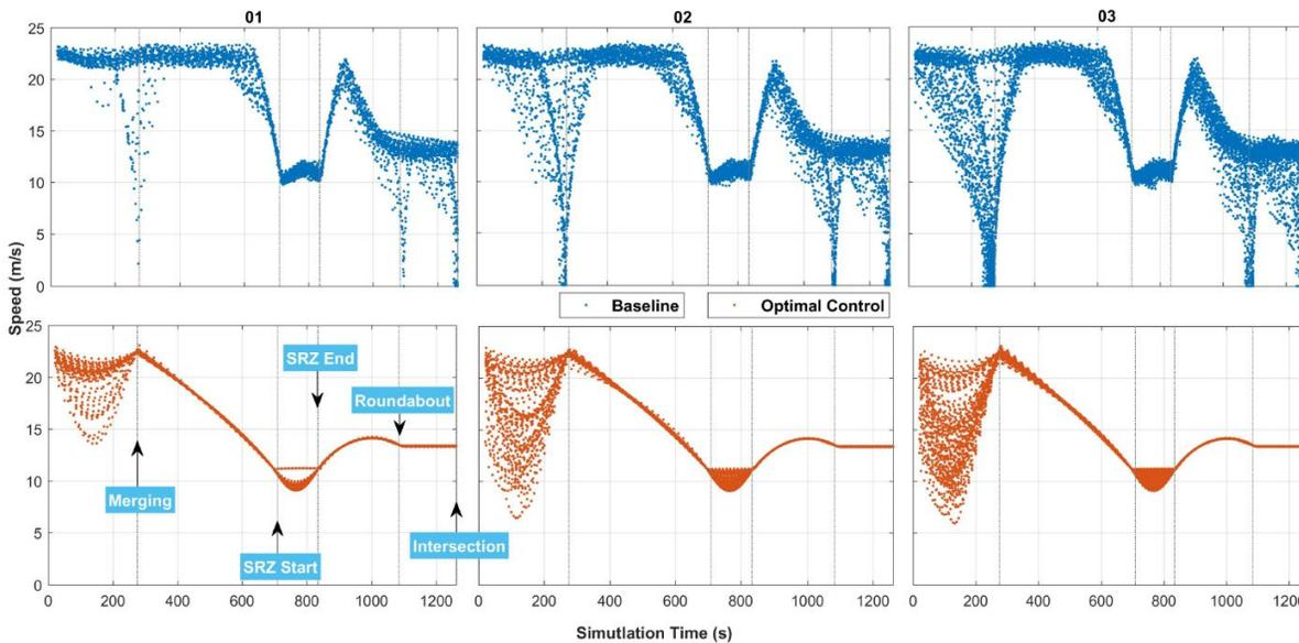
Figure 3-118. Speed profiles for the vehicles in the urban corridor under different scenarios.
