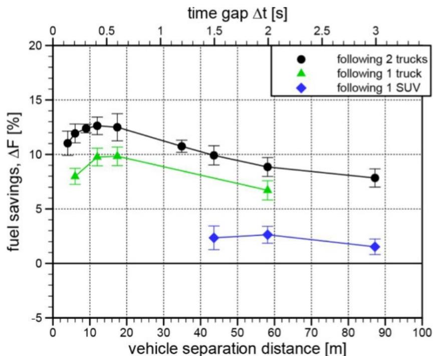
Figure 3-2. Fuel savings of single truck with ACC following an SUV compared to following trucks in two and three vehicle platoons (105 km/h vehicle speed, 29,500 kg vehicle mass).
