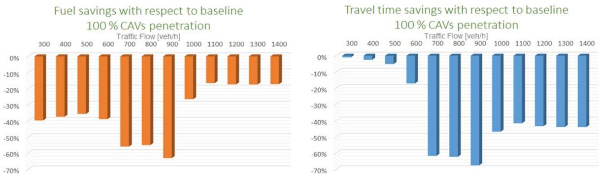
Figure 3-108. System-level fuel consumption (left) and travel time (right) savings for different traffic demands (traffic flow volume was the same on the main and ramp roads).
