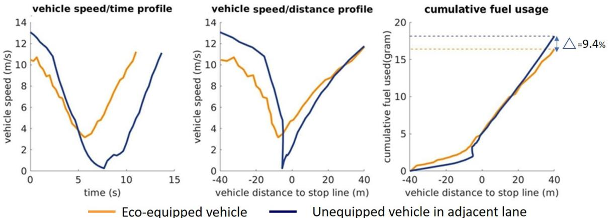
Figure 3-24. Case of Scenario 1: EAD Case I: An eco-equipped vehicle slows down but does not make a full stop. Unequipped vehicle in adjacent lane makes nearly a full stop
