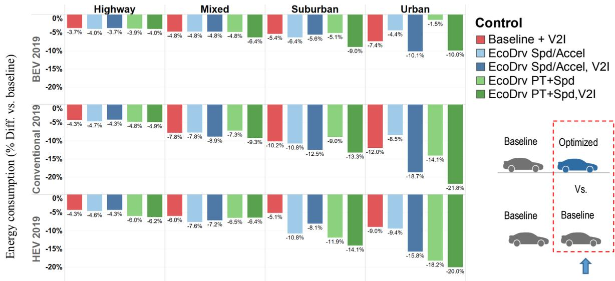
Figure 10. Energy consumption savings compared to baseline control for a vehicle in the lead position, with current powertrain technology, for various powertrains.
