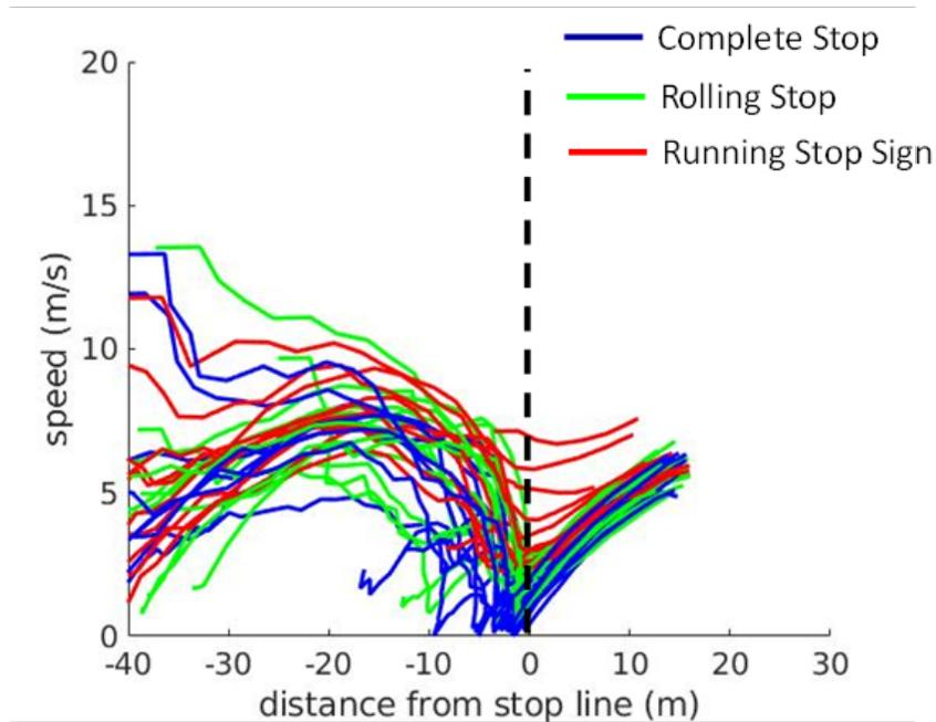
Figure 3-26. Speed profile of the vehicles. Dashed line marks location of the stop sign.
