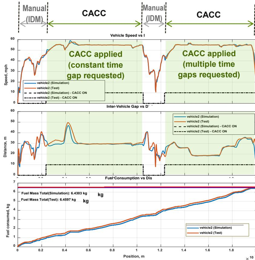
Figure 3-79. Speed, inter-vehicle gap and fuel consumption for middle vehicle in platoon, in test and in simulation
