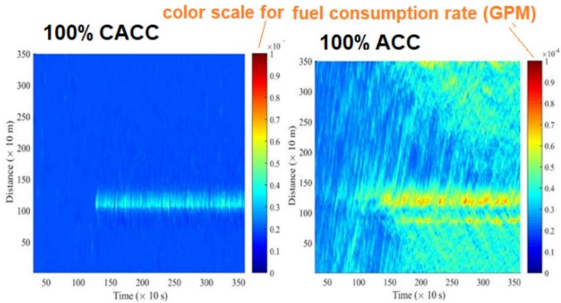
Figure 8. Fuel consumption rate (GPM - gallon per mile travelled) contour plot for 100% CACC driving (left) and 100% ACC driving (right) in response to a traffic disturbance caused by an on-ramp.
