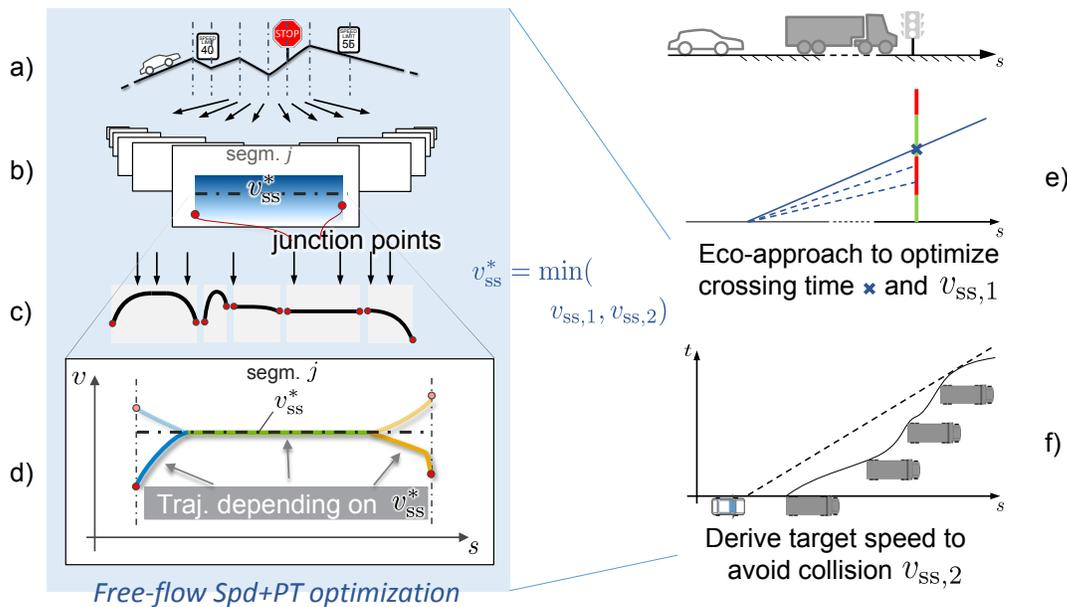
Figure 3-85. The speed+powertrain eco-driving algorithm combines eco-approach to connected traffic lights, collision avoidance, and free-flow optimization.
