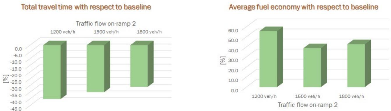
Figure 3-120. Average fuel economy and travel time results for the simulated highway corridor (2.5 km).
