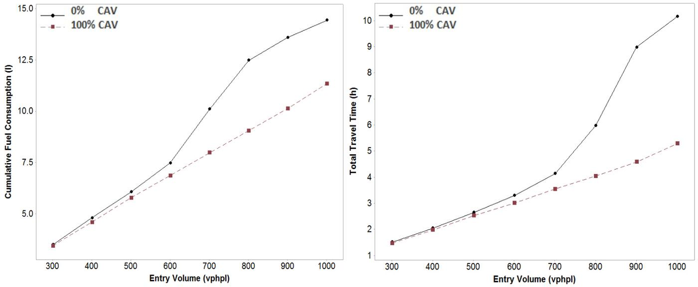
Figure 3-114. Total fuel consumption and total travel time vs. entry volume.
