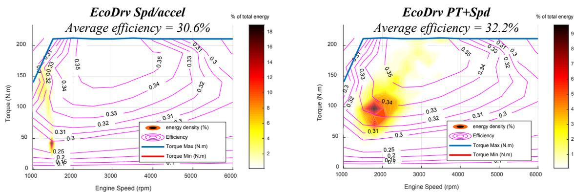
Figure 3-96. Engine operating points (density as a percentage of total energy) for a HEV (current technology) in lead position, for speed-only (left) and speed+powertrain (right) eco-driving strategies in one urban driving example.
