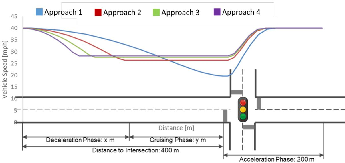
Figure 3-15. Intersection eco-approach and launch with no stop required (Scenario 1).
