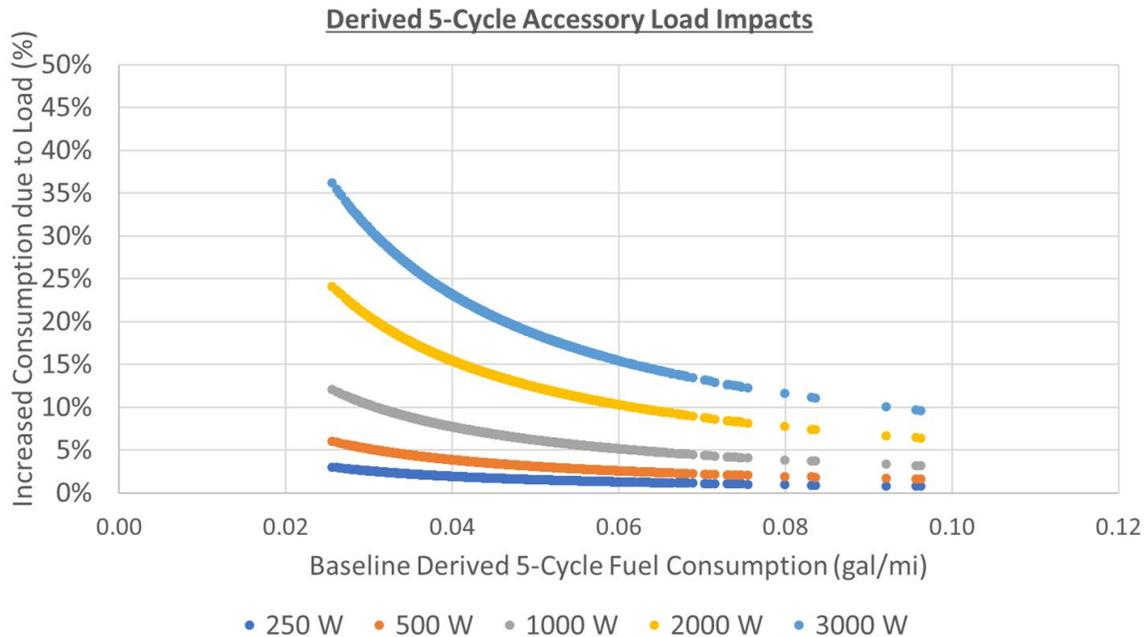
**Figure 3-34. MY2019 ICE vehicle estimated real-world additional electrical load sensitivity.**
