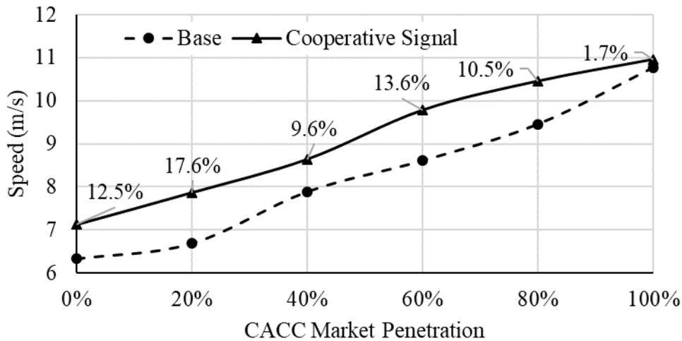
**Figure 3-102. Average vehicle speed at an urban signalized intersection under various CACC market penetrations with and without cooperative signal controller.**
