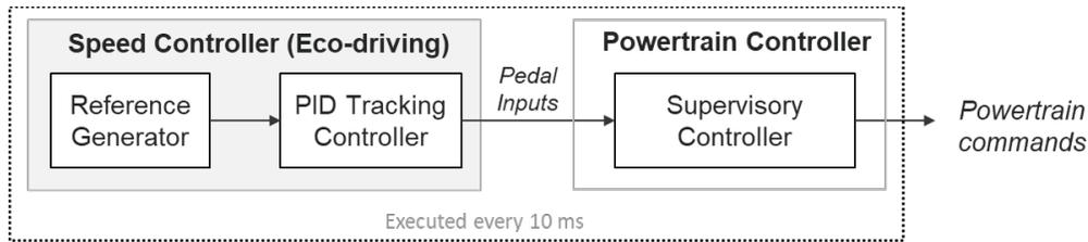
Figure 3-88. Speed and powertrain control architecture in the speed-only eco-driving case.
