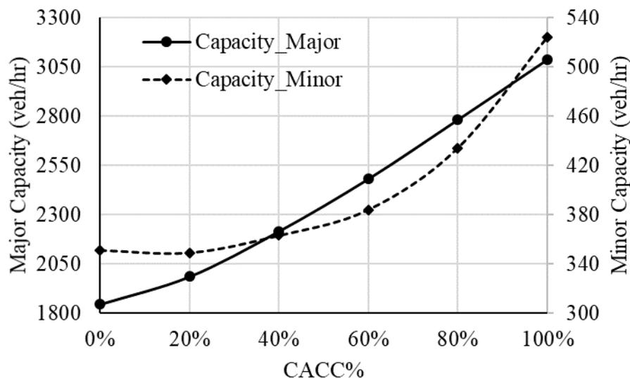
**Figure 3-101. Capacity impact of CACC on an urban signalized intersection without a cooperative signal controller.**
