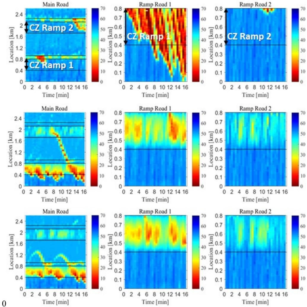
Figure 3-121. Spatial-temporal distribution of mean speed plots of main and ramp roads. Top: 0%, middle: 60% and bottom: 80%.
