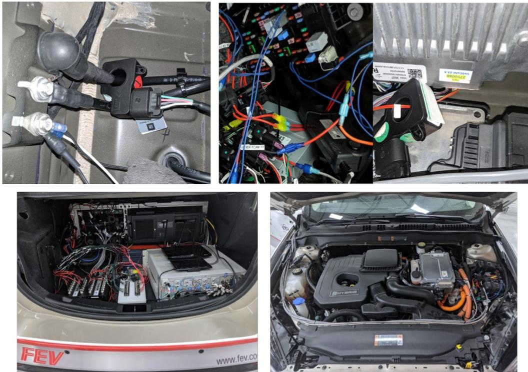
Figure 3-35. Examples of advanced driver-assistance system instrumentation and sense points.
