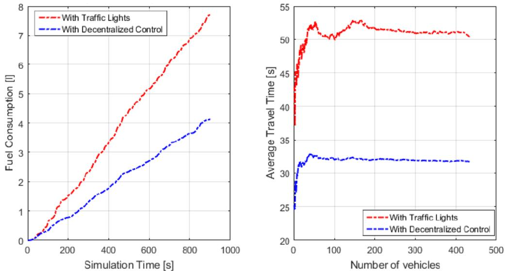
Figure 3-116. Fuel consumption and average travel time improvement for the 434 vehicles passing through the simulated intersections. East-west and west-east corridors were 440 m and 425 m long, respectively.
