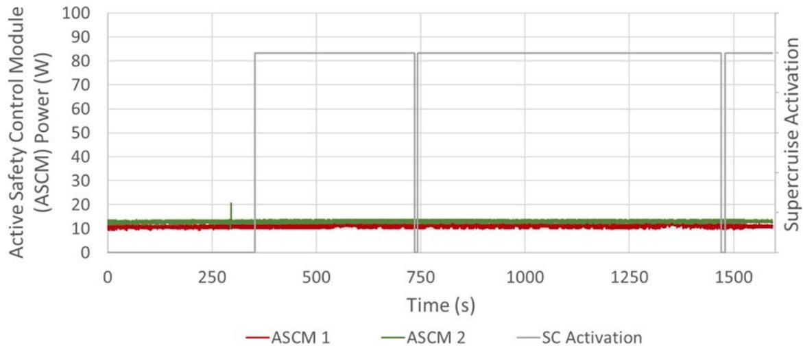
Figure 3-40. Cadillac CT6 active safety control module power consumption during vehicle operation.
