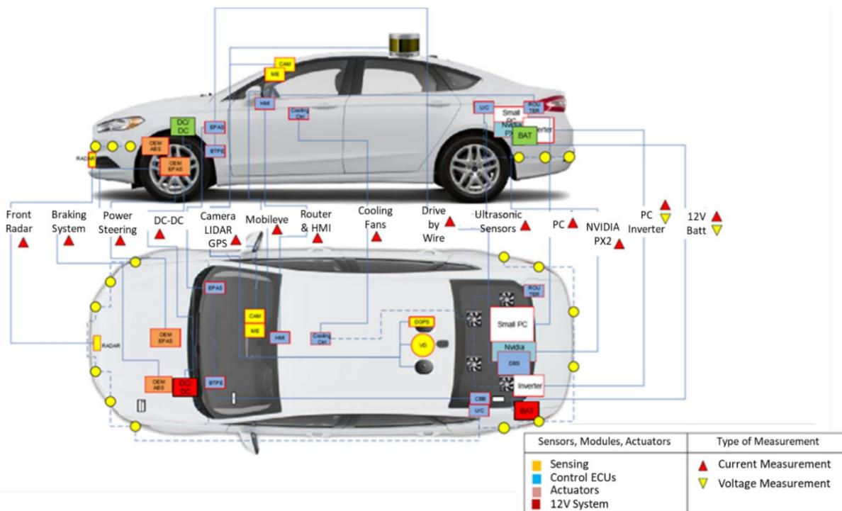
Figure 3-37. Ford Fusion HEV (FEV AV Demonstrator) Instrumentation Overview.
