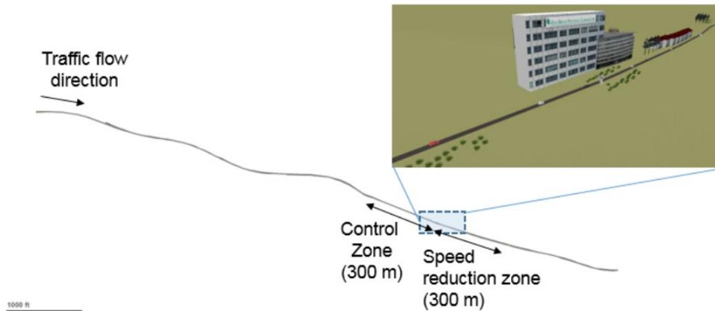
Figure 3-105. Traffic network developed in Vissim for the speed harmonization case.
