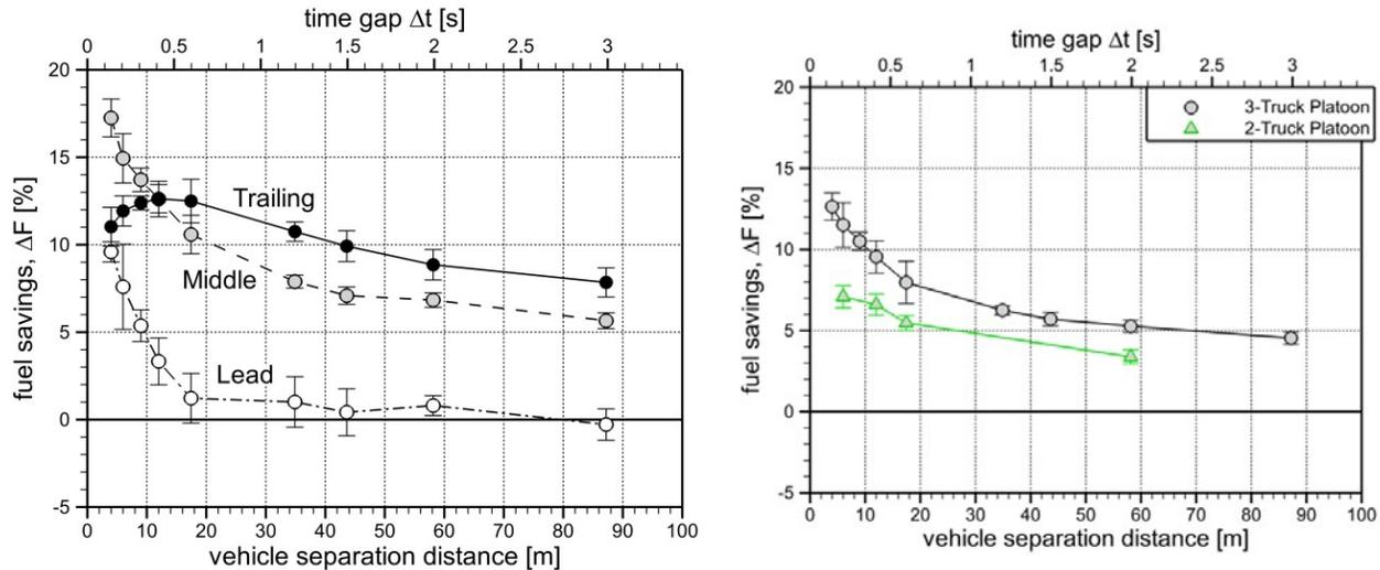
Figure 3-1. Fuel savings for individual trucks as a function of separation distance (left) and average fuel savings for two- and three-truck platoons (right).
