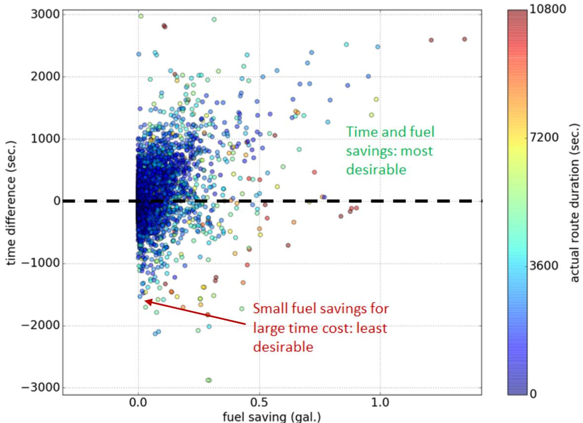
Figure 3-29. Energy savings vs. time savings for alternative routes compared to actual routes.
