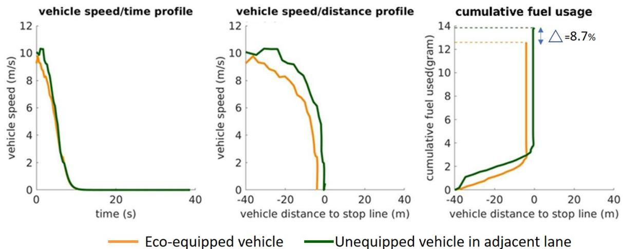
Figure 3-22. EAD Scenario 2: Eco-equipped and unequipped vehicles travel in adjacent lanes and arrive at intersection at a similar time.
