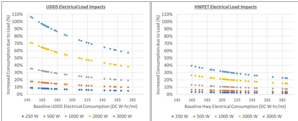
**Figure 3-31. Baseline highway electrical consumption for MY 2019 BEVs and their estimated UDDS and HWFET energy consumption sensitivities.**
