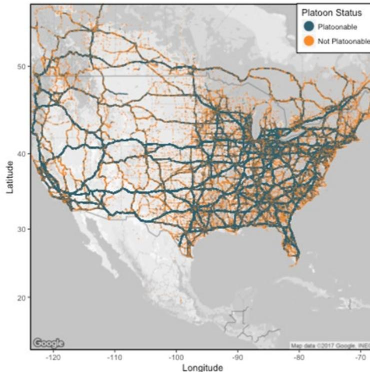
**Figure 2. Snapshot of US platoonability based on partner analysis for a single day. Observations with speeds less than 30 mph are omitted for clarity.**
