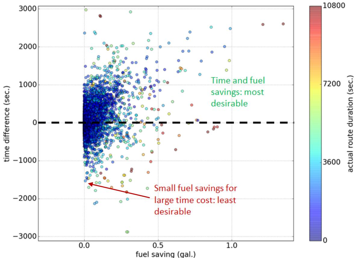
Figure 5. Energy savings vs. time savings for alternative routes compared to actual routes.
