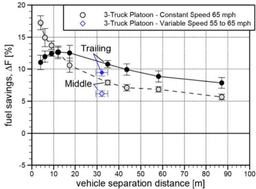
Figure 3-4. Middle and trailing vehicle fuel-savings results for three-vehicle CACC tests with 1.2 s separation time and speed variation (89 to 105 km/h), with changes in speed every 100 seconds. Horizontal error bars represent range of separation distances (29,500 kg vehicle mass).
