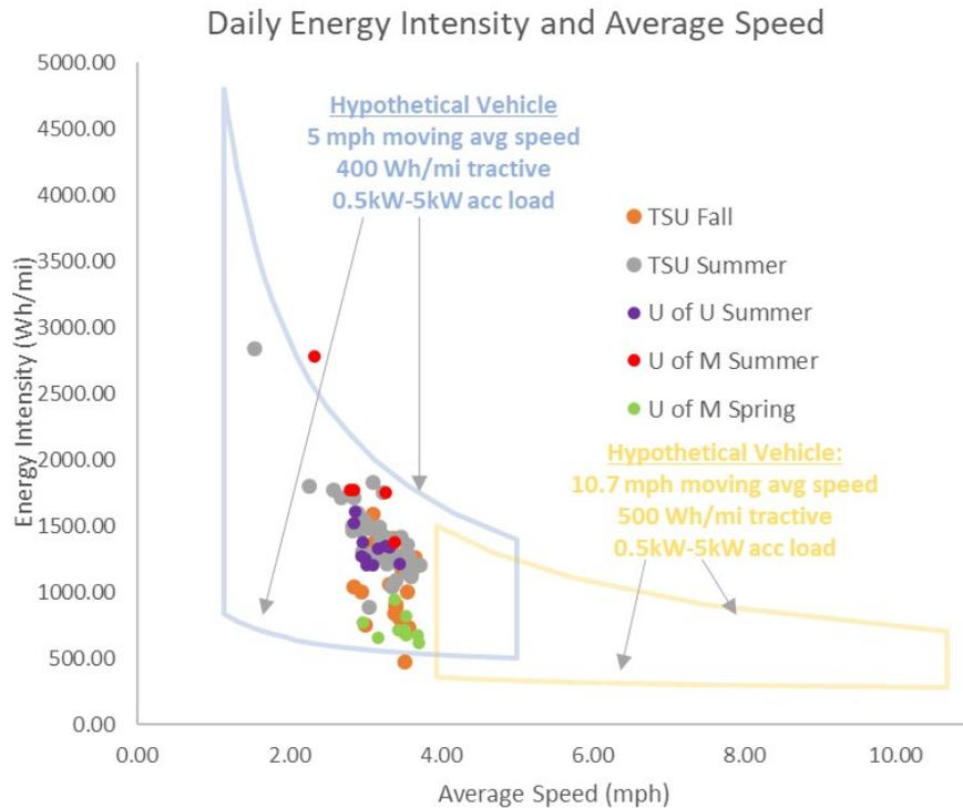
**Figure 3-53.** Daily energy intensity of each pilot shown relative to average daily speed, along with illustrated ranges of a simple hypothetical vehicle.
