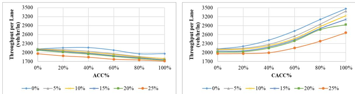
Figure 7. Corridor throughput versus ACC penetration level (left) and CACC penetration (right); the color codes represent the percent flow through the off-ramp with respect to the mainline volume.
