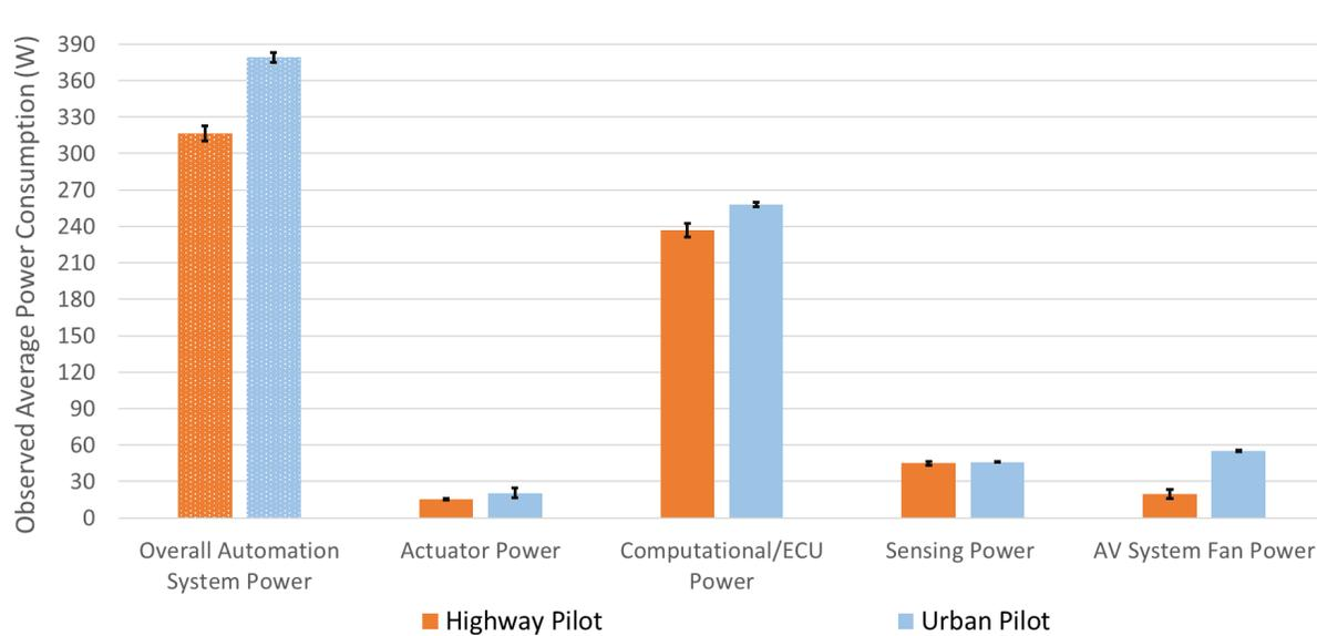
Figure 3-41. FEV Smart Demonstrator automation electrical loads during Highway Pilot and Urban Pilot operation on public roads (95% confidence interval shown in error bars).
