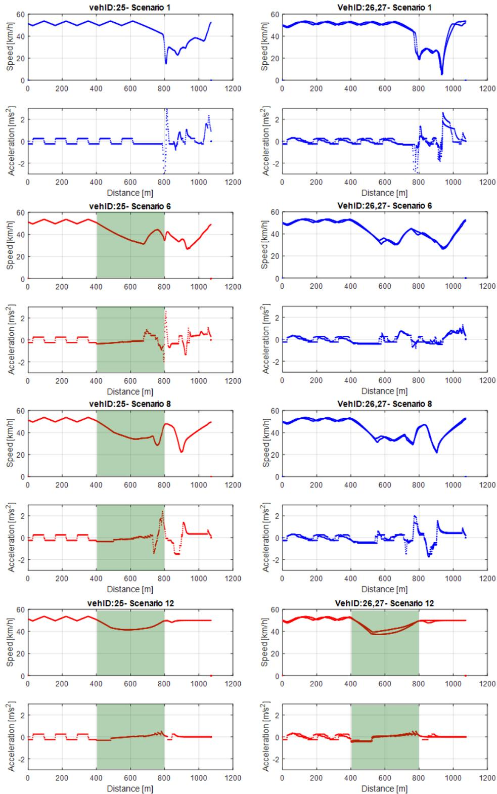
Figure 3-111. Speed and acceleration profiles for three consecutive vehicles in scenarios 1, 6, 8 and 12 described in Table 3-14.
