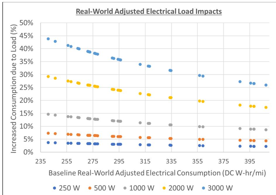
Figure 3-32. Estimated real-world consumption sensitivity to additional electrical loads for MY2019 BEVs.
