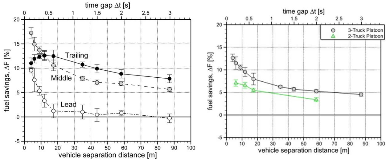
**Figure 1. Fuel Savings for Individual Trucks as a Function of Separation Distance (left) and Average Fuel Savings for Two- and Three-Truck Platoons (right).**
