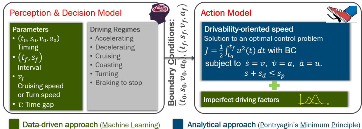
Figure 3-81. Schematic diagram of the human driver model: perception & decision model (left) and action model (right).
