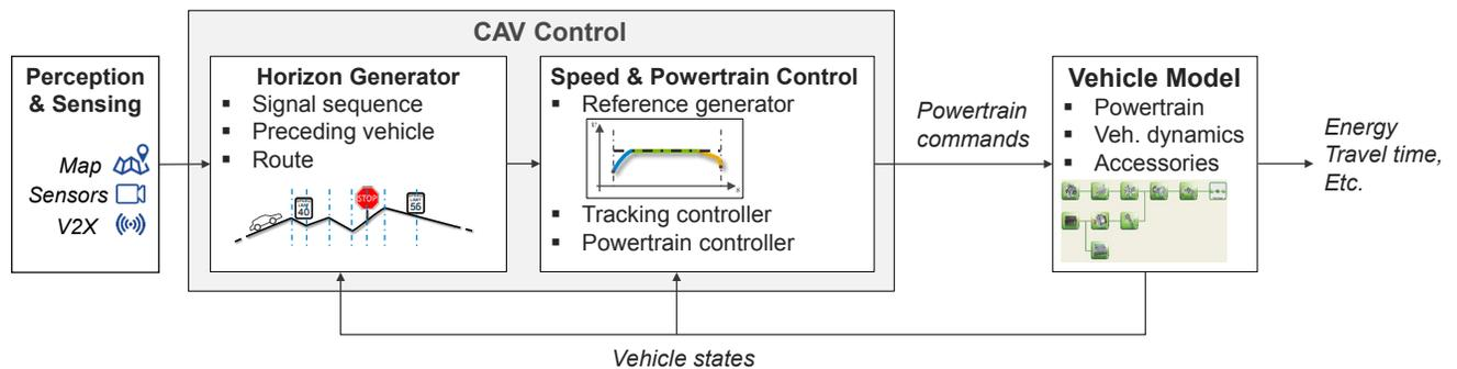
Figure 3-87. Architecture of the CAV controller.
