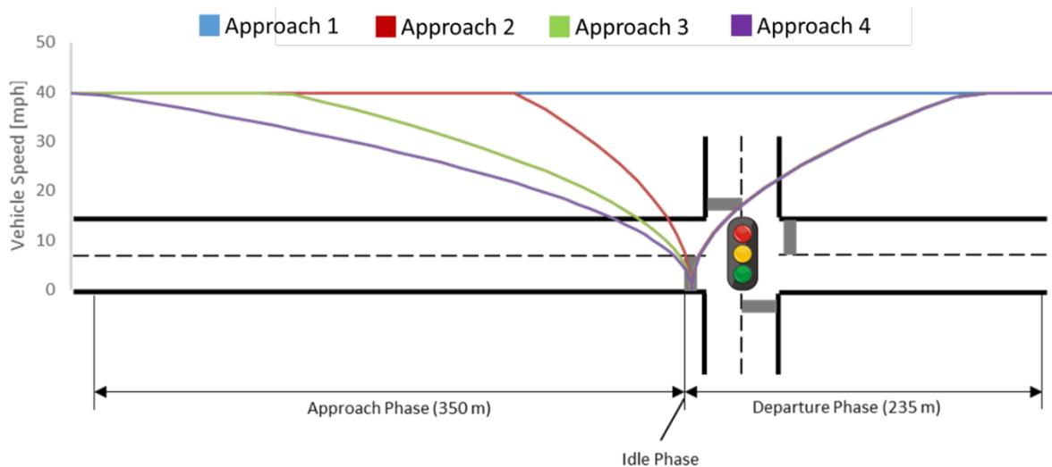
Figure 3-17. Intersection eco-approach with stop and idle required (Scenario 2).
