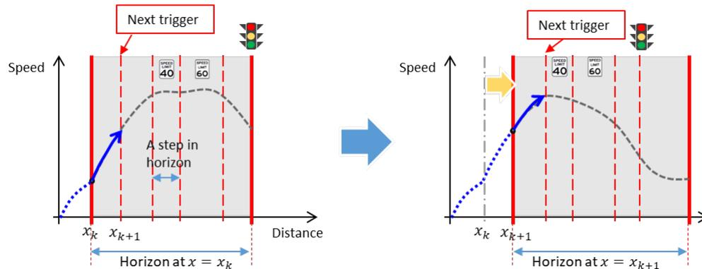
Figure 3-86. Concept of receding horizon: The prediction window at position  $x_k$  (left) advances at the following step,  $x_{k+1}$  (right).
