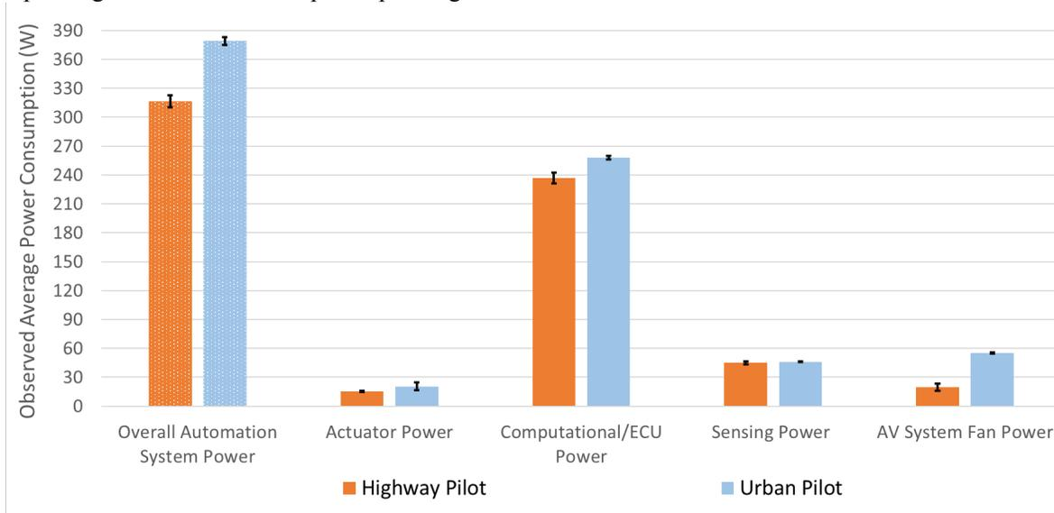
**Figure 6.** FEV Smart Demonstrator automation electrical loads during Highway Pilot and Urban Pilot operation on public roads (95% confidence interval shown in error bars).
