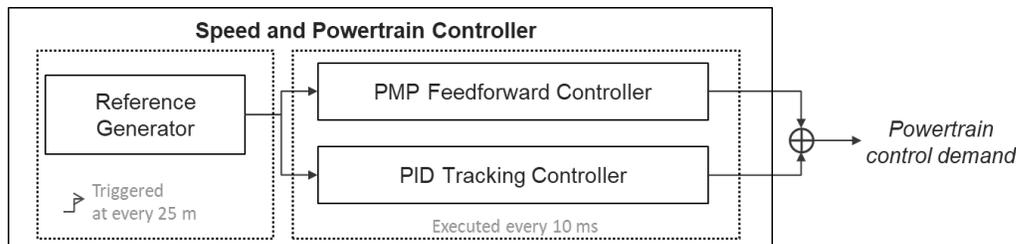
Figure 3-89. Speed and powertrain control architecture in the speed + powertrain eco-driving case.
