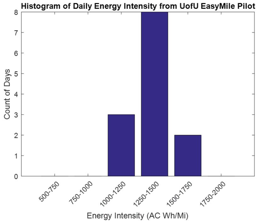
Figure 3-50. Distribution of U of U EasyMile shuttle energy intensity.
