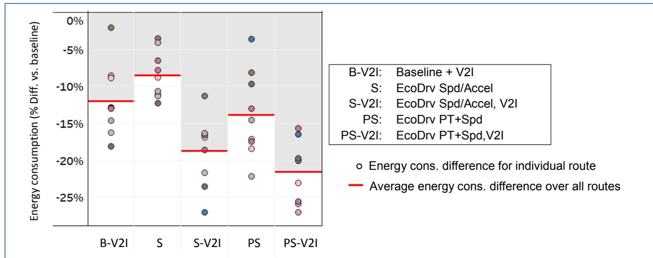
Figure 3-99. Distribution of energy savings for lead vehicle (conventional, current technology, urban scenarios).
