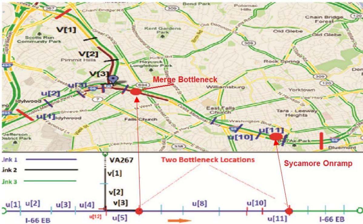
Figure 3-100. Road geometry for microscopic traffic simulation: I-66 EB inside the Beltway, with two bottlenecks marked with red spots.
