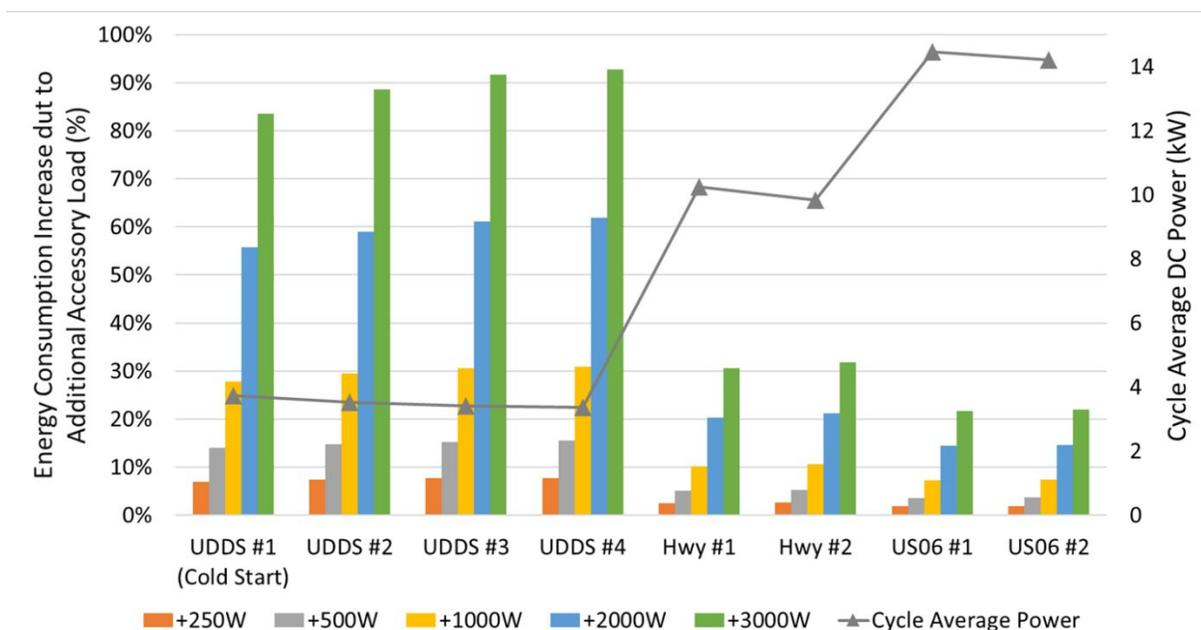
Figure 3-30. Chevrolet Bolt estimated additional load sensitivity and cycle average energy consumption for U.S. regulatory cycles.
