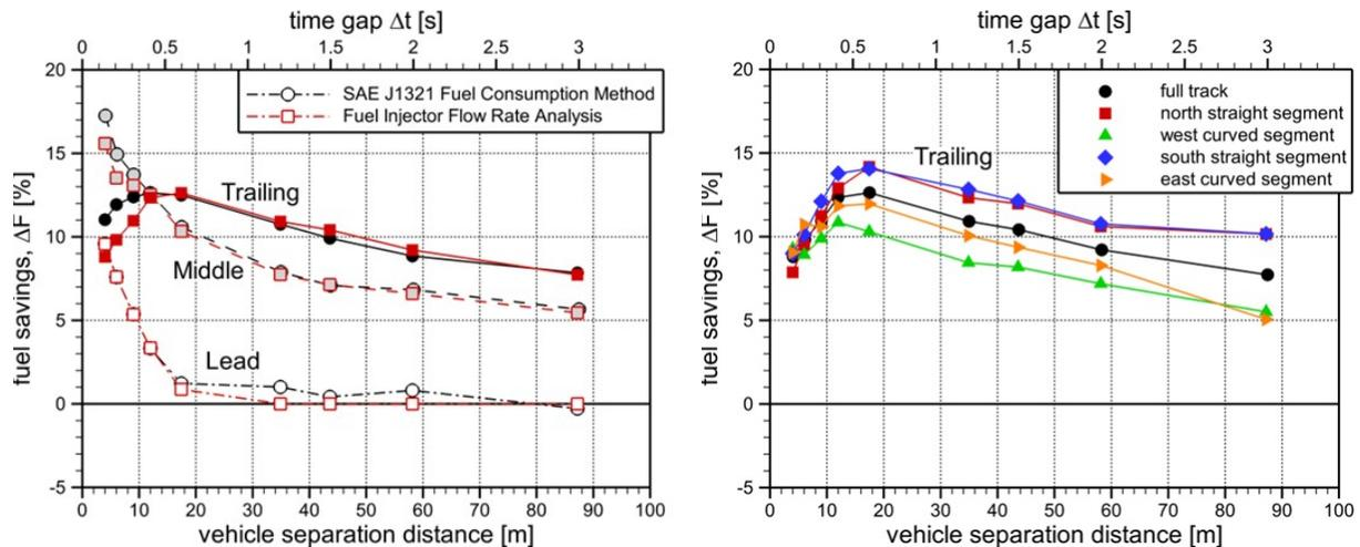
Figure 3-5. (Left) Comparison of J1321 fuel weighing and CAN bus showing fuel injector signal measurements of fuel consumption and (right) CAN bus fuel injector measurements delta fuels savings on straight and curved track.
