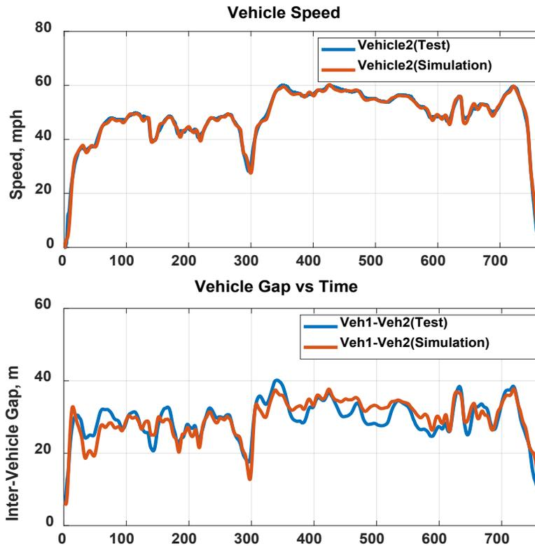
Figure 3-80. Comparison of the ACC model in RoadRunner with test data from the chassis dynamometer. Vehicle 1 is driven by a human. Vehicle 2 is outfitted with the ACC system.
