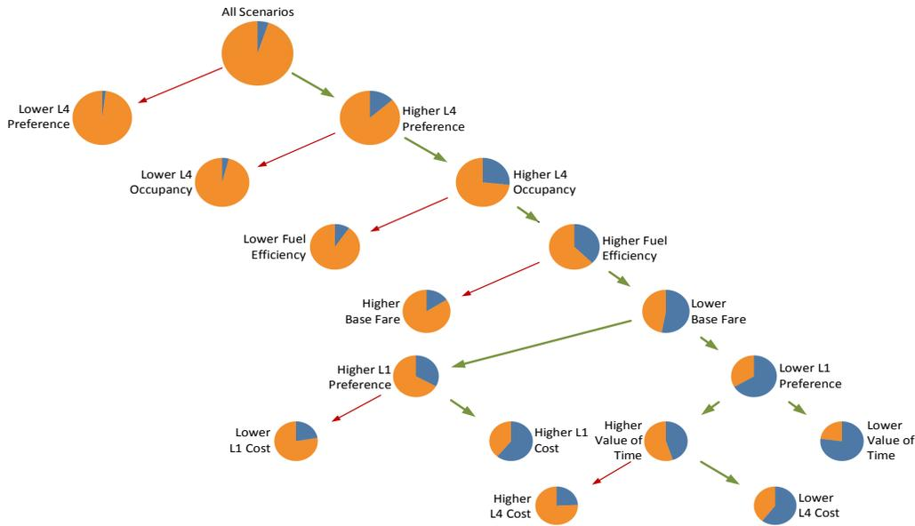
**Figure 3-72. Regression tree (for the energy study) showing major influences on energy consumption from tipping points scenario modeling efforts; dark blue in each pie chart indicates the fraction of scenarios that lie in the best 5% of fuel consumption, within simulations selected by the preceding branching criterion.**
