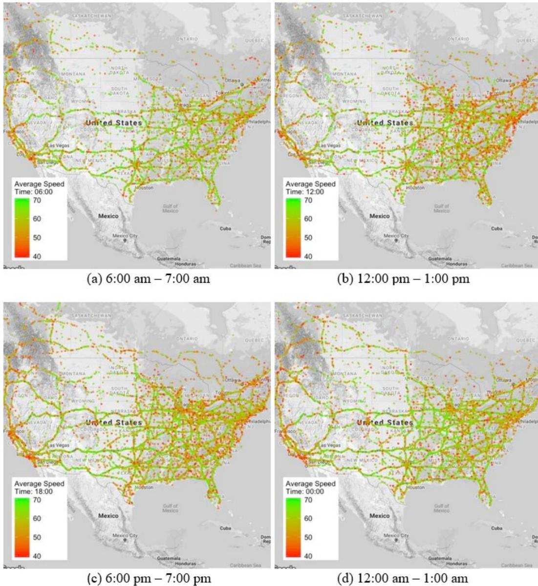
Figure 3-10. Geographic representation of hourly average speed at different times of day.
