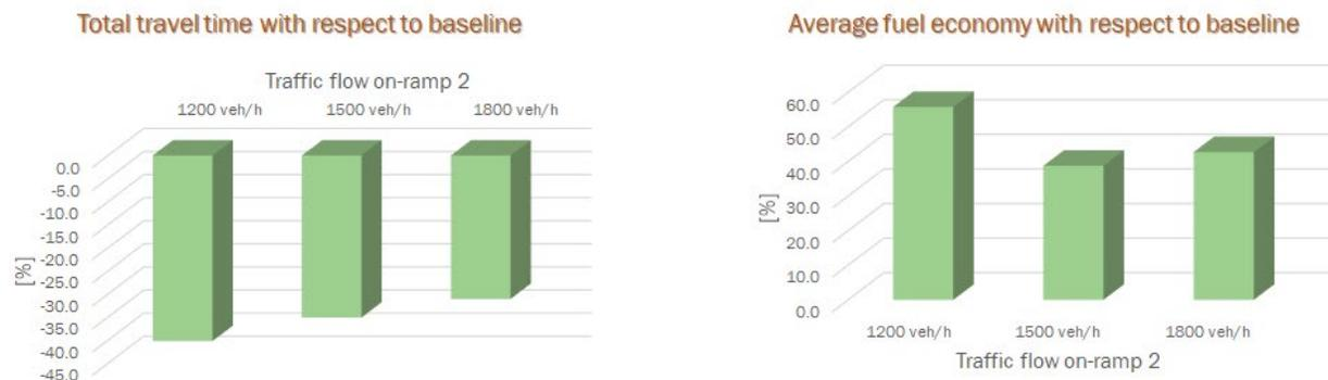
Figure 12. Average fuel economy and travel time results for the simulated highway corridor (2.5 km).
