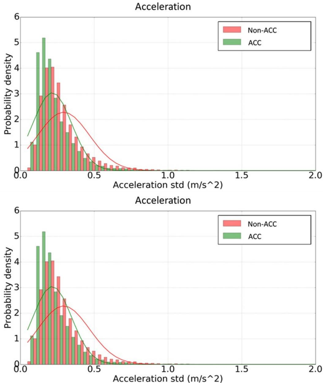
Figure 3-13. Distributions of acceleration (top) and deceleration (bottom) standard deviations in ACC and non-ACC mode.
