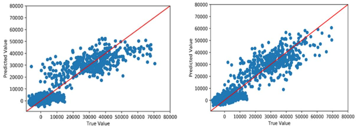
**Figure 3-74. Predicted values of average daily traffic (ADT) flows vs true values for the KNN model (a) and the RF model (b).**
