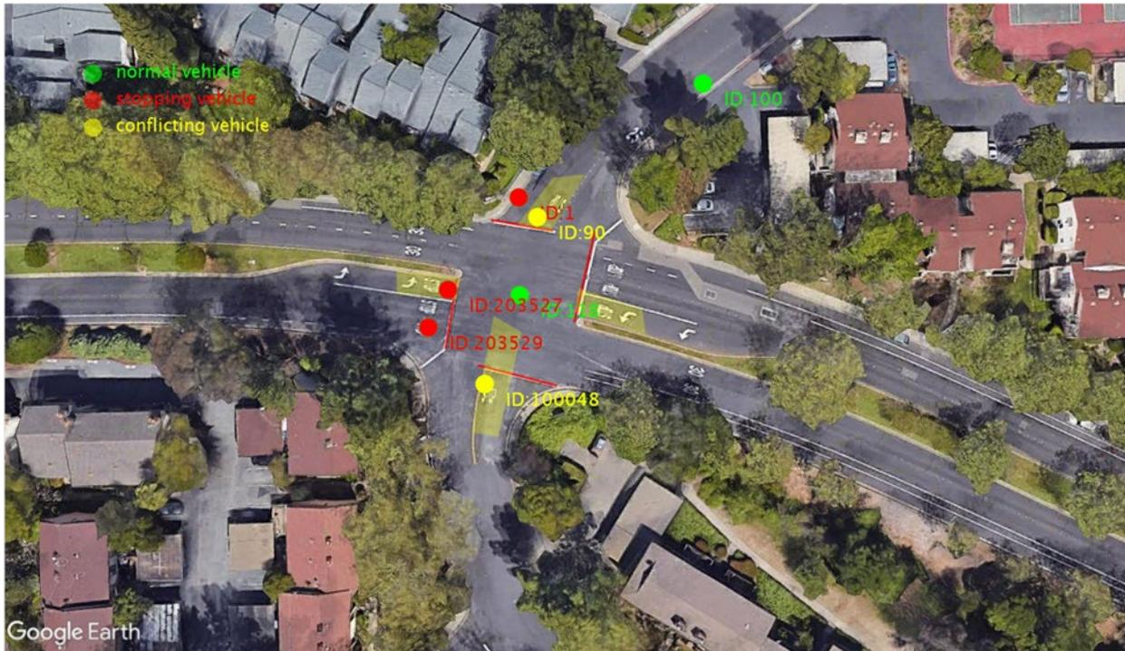
Figure 3-25. Unsignalized intersection in Pleasant Hill with mapped vehicle detections.
