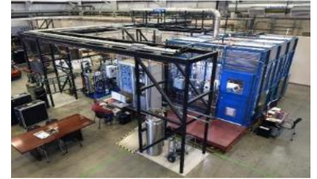
25 kW high-temperature electrolysis @ INL Energy Systems Laboratory
