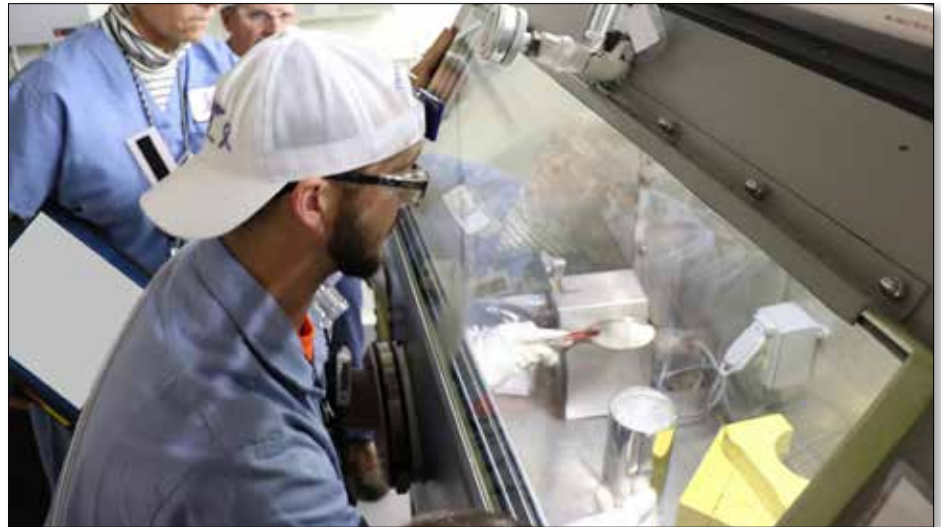
Workers with Isotek Systems use gloveboxes to safely open canisters and handle hazardous materials in the downblending process of U-233 stored at Oak Ridge National Laboratory.
