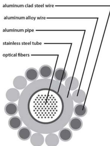
Figure 1: OPGW Cross-Section
