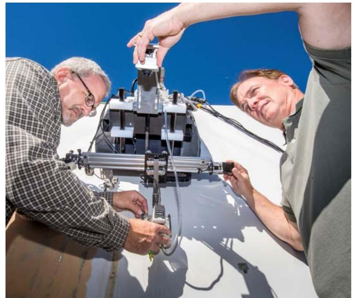
Tom Rice, left, and Dennis Roach, right, of Sandia National Laboratories set up a crawling robot to inspect a wind turbine blade segment. Photo: Randy Montoya, Sandia National Laboratories
