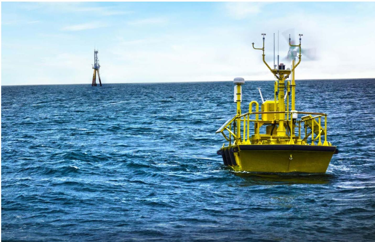
Buoys stationed off U.S. coasts collect meteorological and oceanographic data that can help the wind industry make informed decisions for offshore wind power plants. Feedback from industry spurred instrument upgrades that will help provide more meaningful data. *Photo by Ocean Tech Services, LLC, and PNNL*
