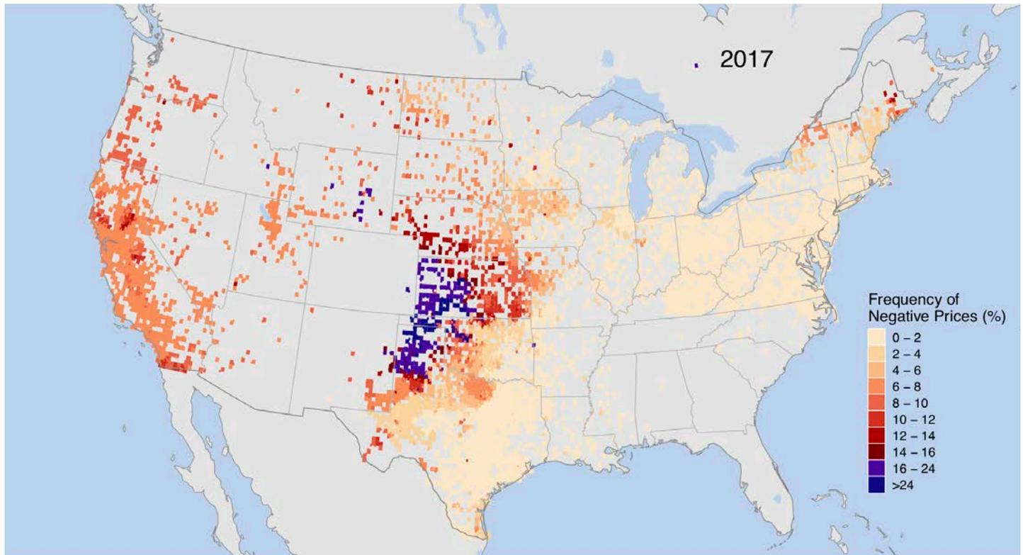
Figure 1. Frequency of negative locational marginal prices (LMPs), or real-time power prices, in 2017. This analysis determined that areas with high levels of wind and solar increased the frequency of negative prices. *Figure by Lawrence Berkeley National Laboratory*
