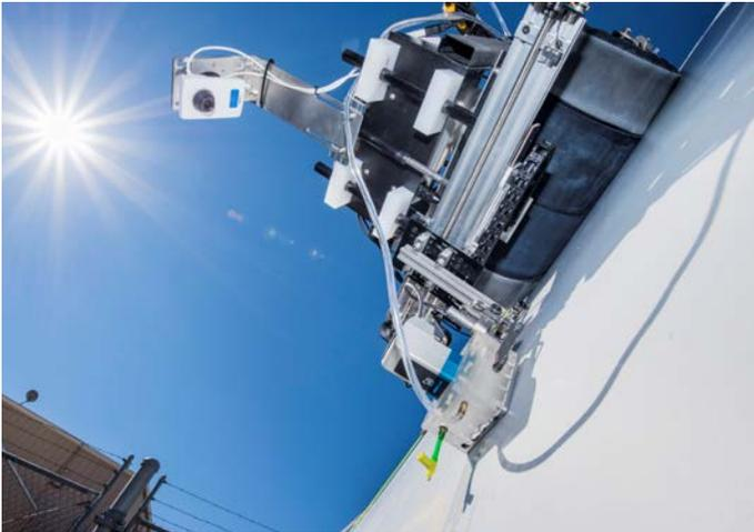
Sandia National Laboratories researchers use crawling robots and drones with infrared cameras to look for hidden damage to keep wind turbine blades operating longer and drive down the costs of wind energy. Photo: Randy Montoya, Sandia National Laboratories
