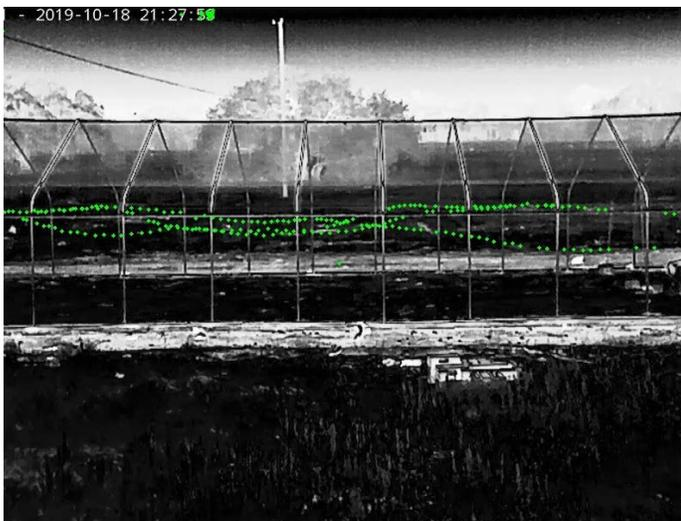
Preliminary field trials have demonstrated a new flight tracking method capable of measuring how various bat species behave in the presence of ultrasonic acoustic deterrents. The green dots show the flight track of an individual bat. The researchers must use four thermal camera images like the one shown here to cover the entire length of the flight cage. *Image by Brittany Stamp, Texas State University*
