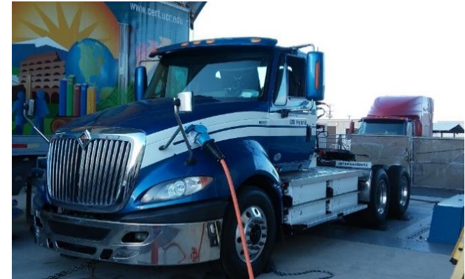
US Hybrid eTruck™ #1 layout with EnerDel battery pack 180kWh (11 packs)
