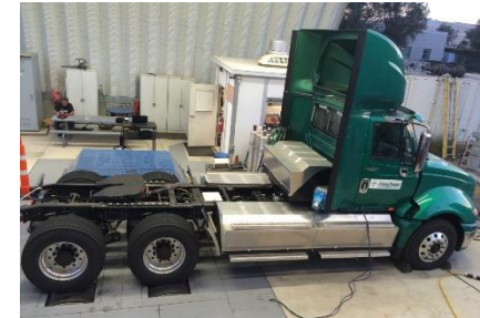
EDD-2 undergoing testing on UC Riverside chassis dynamometer.
