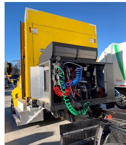
TransPower PHET No. 2 rear view showing APU
