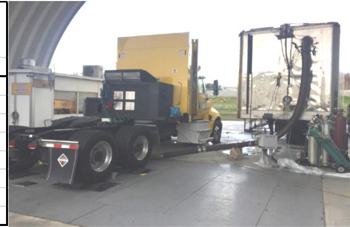
TransPower PHET No. 2 at UCR's heavy duty chassis AC transient dynamometer
