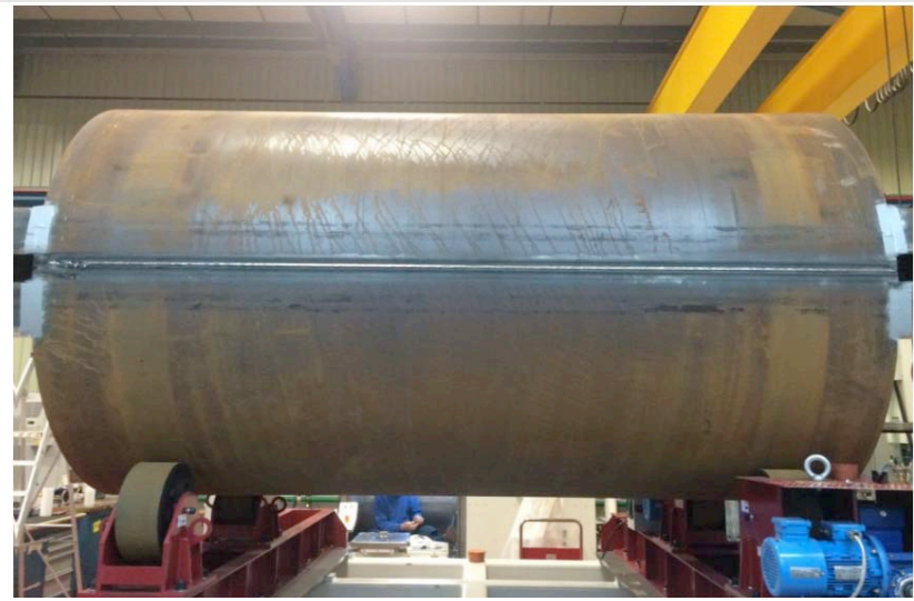
65mm (thick) x 3m length x 1.8m diameter Welding time: <10 minutes
