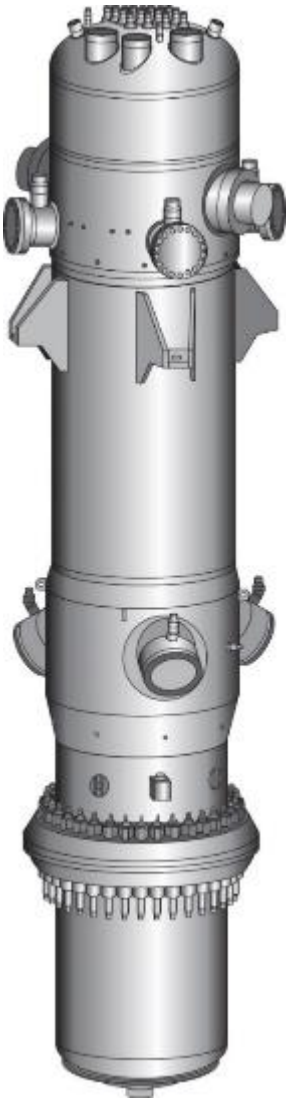
Representative Model of NuScale Power Reactor Vessel
