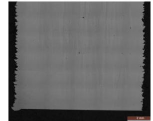
Optical Image Showing Crack Free Walls
