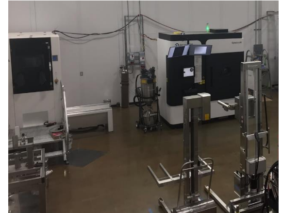
Arcam Spectra H Installed at ORNL-MDF
