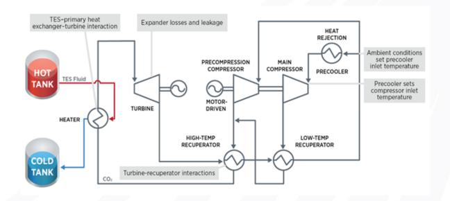
RCBC integrated with thermal energy storage at ~550°C for Integrated TESTBED FOA
