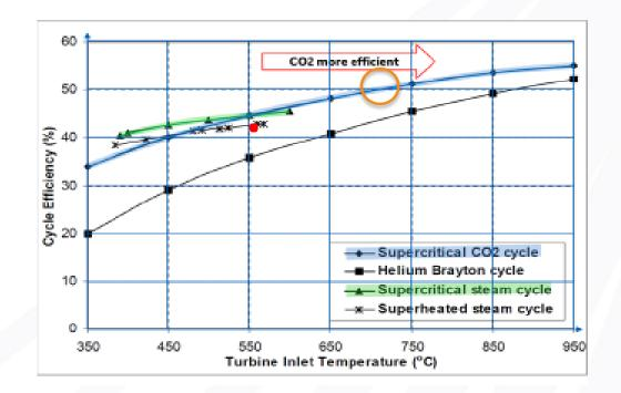
More efficient than steam cycle in 540-750°C Turbine Inlet Temperature
