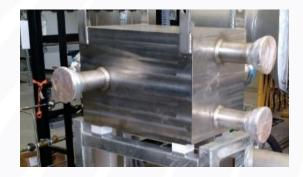
Robust in operation, but less than optimal effectiveness (~80%, 92% target)
