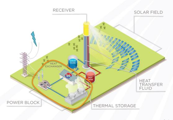
Target: 50% Efficiency at 715°C turbine inlet temperature at 900 \$/kWE, air cooling
