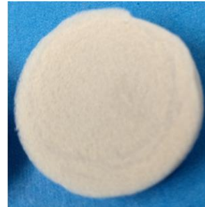
Slab made by crosslinking particles ( k \approx 0.018 \text{ W/m.K} )
