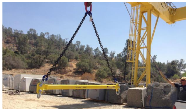
Photo 4. Example of a spreader bar used for hoisting and rigging
