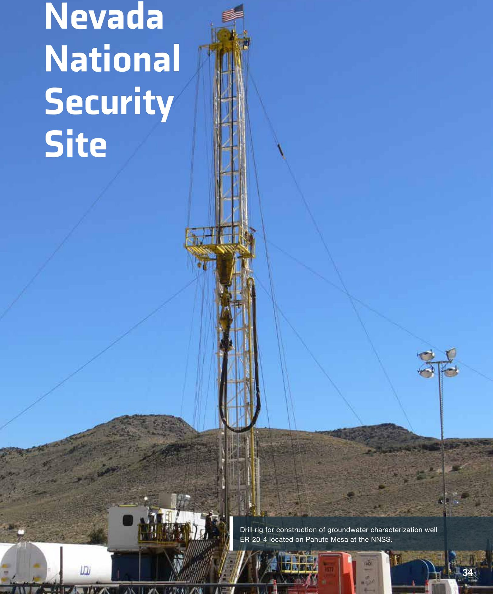
Drill rig for construction of groundwater characterization well ER-20-4 located on Pahute Mesa at the NNSS.
