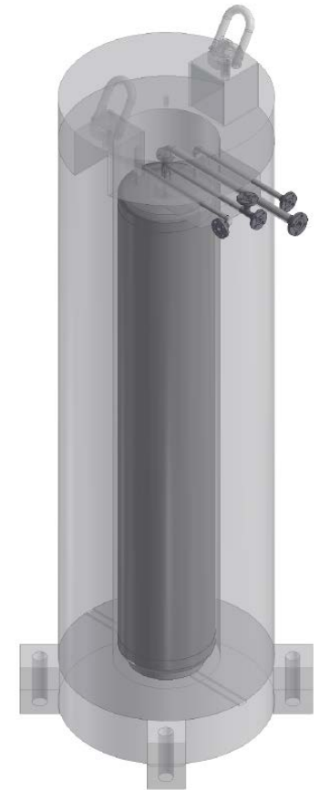
Shielded Ion Exchange Column (Dimensions 12'x5.5' Shielded)
