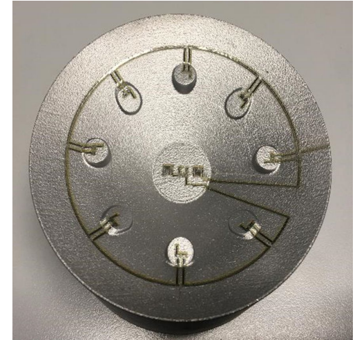
Printed electronics test structure (~ 4" dia. X 5" height, 0.25" wall thickness)
