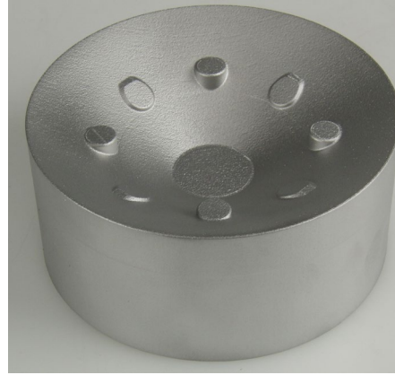
Printed electronics test structure (~ 4" dia. X 5" height, 0.25" wall thickness)
