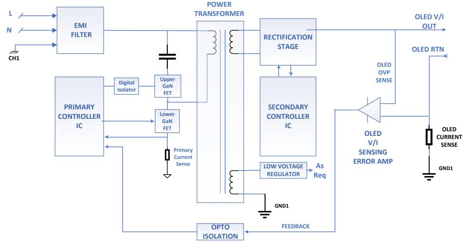
Active Clamp Flyback - OLED High Efficiency Driver Block Diagram
