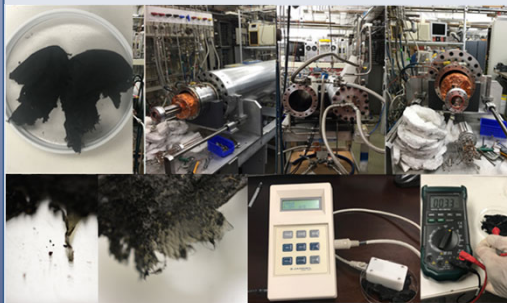
Figure 3. Photographic images of CNT TCF (top left) from HiPICO reactor filter (top right), zoomed images of transparent CNT TCF contaminated by carbon dusts (bottom left), resistance characterization (4 \Omega/\square ).
