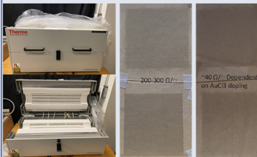
Figure 2. Photographic images of 1200 °C three zone furnace (left), direct deposited CNT TCF without (middle) and with (right) \text{AuCl}_3 doping.
