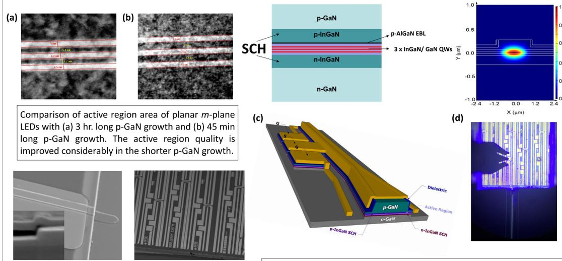
(a) Comparison of active region area of planar *m*-plane LEDs with (a) 3 hr. long p-GaN growth and (b) 45 min long p-GaN growth. The active region quality is improved considerably in the shorter p-GaN growth. (c) Epitaxial layer structure of the SLD indicating the separately-confined heterostructure guiding, whose simulated mode profile using Lumerical (FDTD) is shown in (b). (d) Pictographic illustration of a fabricated tapered waveguide SLD (TSLD). (e) A TSLD under electrical operation.
