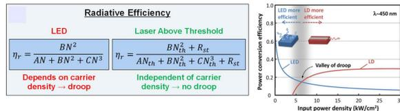
Comparison of the expression for IQE using the ABC model for spontaneous emission dominated devices (LEDs) and stimulated emission dominated devices (SLDs and laser diodes) [J. J. Wierer et al., (2013)]
