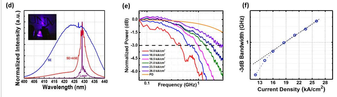
(d) Normalized EL spectra of LED, SLD, and laser on the same chip. (e) Frequency response of the TSLD. The -3 dB RF modulation bandwidth is obtained and plotted versus current density in (f). The  $\log(f_{3dB})$  goes linearly as a function of  $J$  in the superluminescence regime due to the exponential increase of the o/p power with  $J$ , evident from the above equation.
