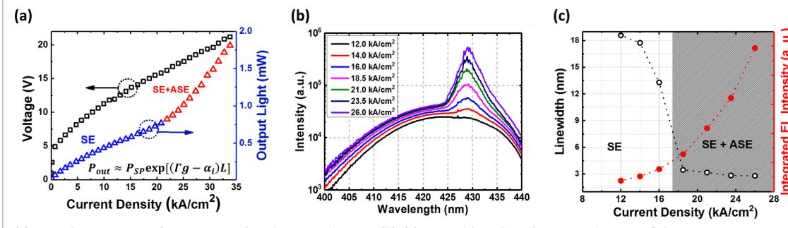
(a) L-J-V characteristics of TSLD. Spectral evolution is shown in (b). (c) Linewidth and total integrated power of the EL spectrum versus current density.
