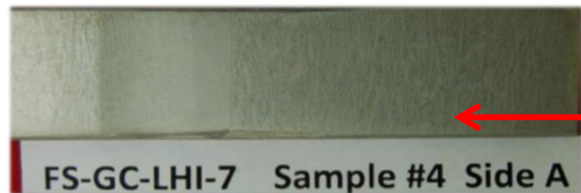
Low-temperature FSW weld (<780°C)
