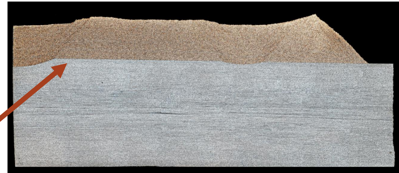
Coupon 2.29: 700 psi, 500°C [~ 5-mm buildup]
