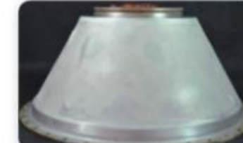
Cold Spray Repaired Reduction Gearbox Housing
