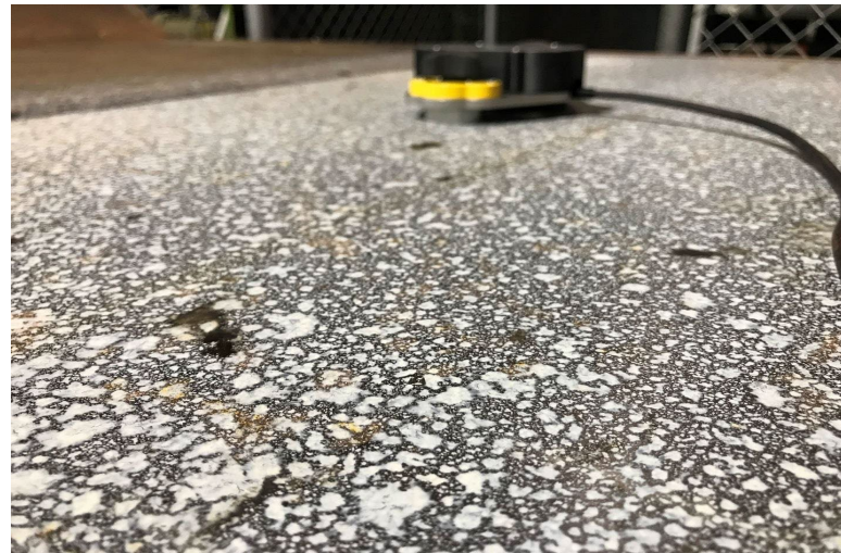
Kaolite dust on the surface of the mockup for the dirt testing.
