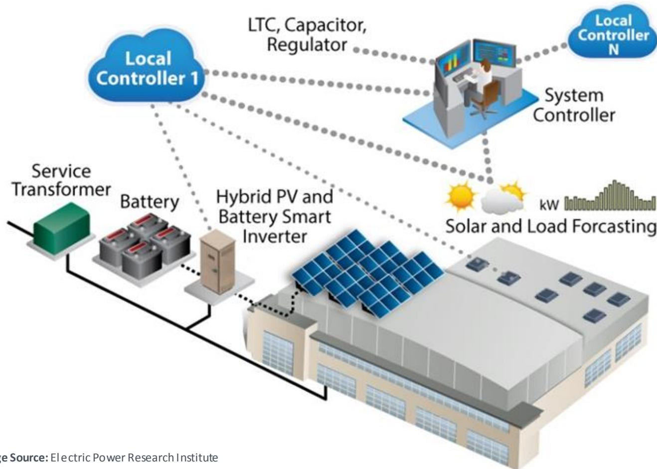
Coordination of controls and enhanced communication capabilities by solar inverters that can restart power on segments of the distribution system (or microgrids) during an outage
