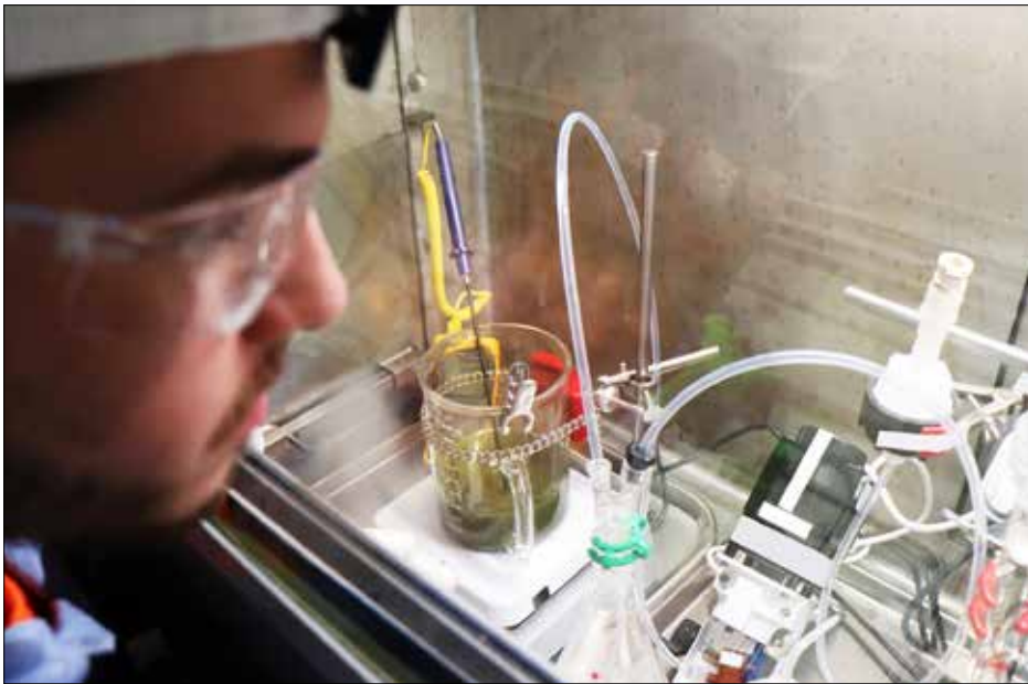
Workers extract thorium from U-233 using a series of gloveboxes to avoid contact with the material or chemicals used in the process. It begins by mixing the uranium with nitric acid.
