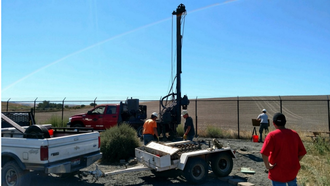
Figure 2-2: Onsite core sample retrieval using a specialized drill rig. Core samples were assessed to complete the geotechnical survey report that informed system design specifications.
