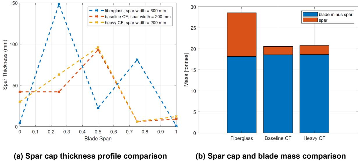
**Figure 4-2. Land-based turbine optimal solution spar cap dimensions.**
