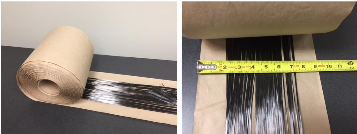
**Figure 2-6. Example of initial heavy-tow CFTF material winding.**
