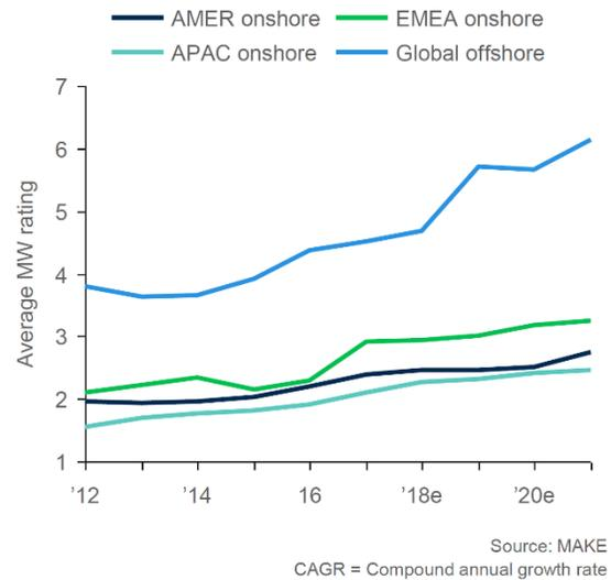
**Figure 1-1. Global trends for wind turbine power rating and diameter increase.**
