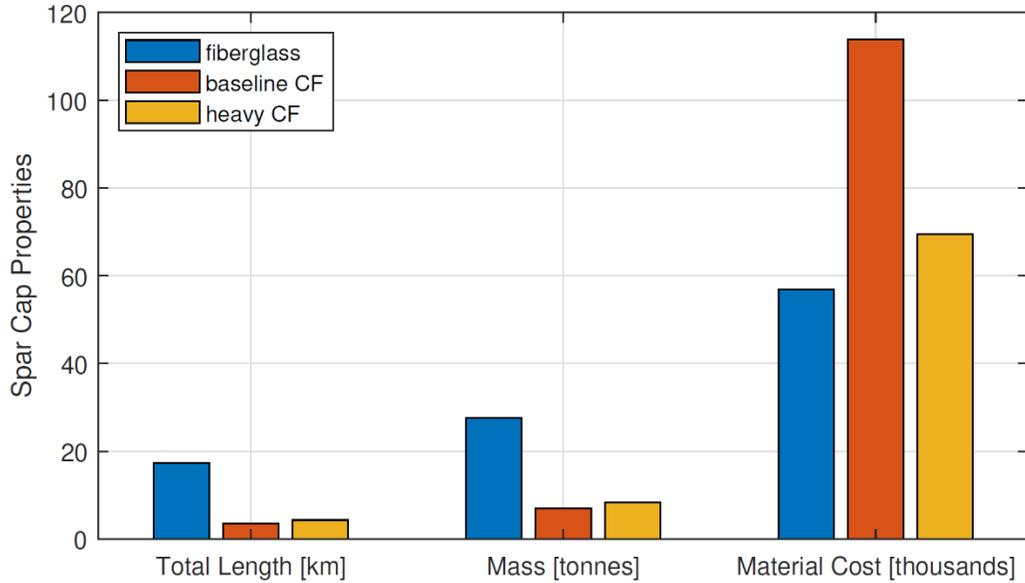
**Figure 4-6. Offshore turbine optimal solution spar cap properties.**
