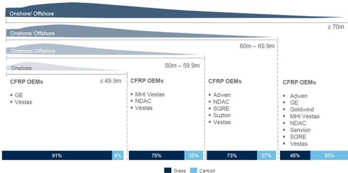
Note: % use of spar material on "current" and "prototype" turbine platforms in the market
