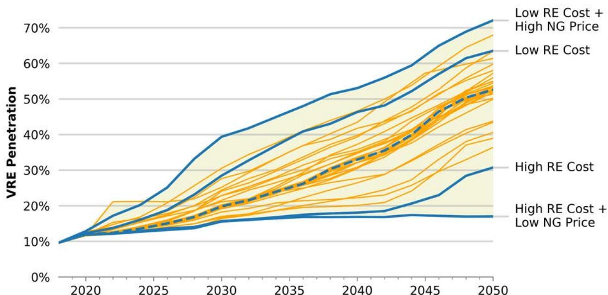
**Figure 12. VRE penetration over time across the suite of scenarios.** The highest and lowest VRE penetration scenarios in 2050 are labeled, along with the Low and High RE Cost scenarios. VRE penetration is defined as VRE generation divided by total generation.
