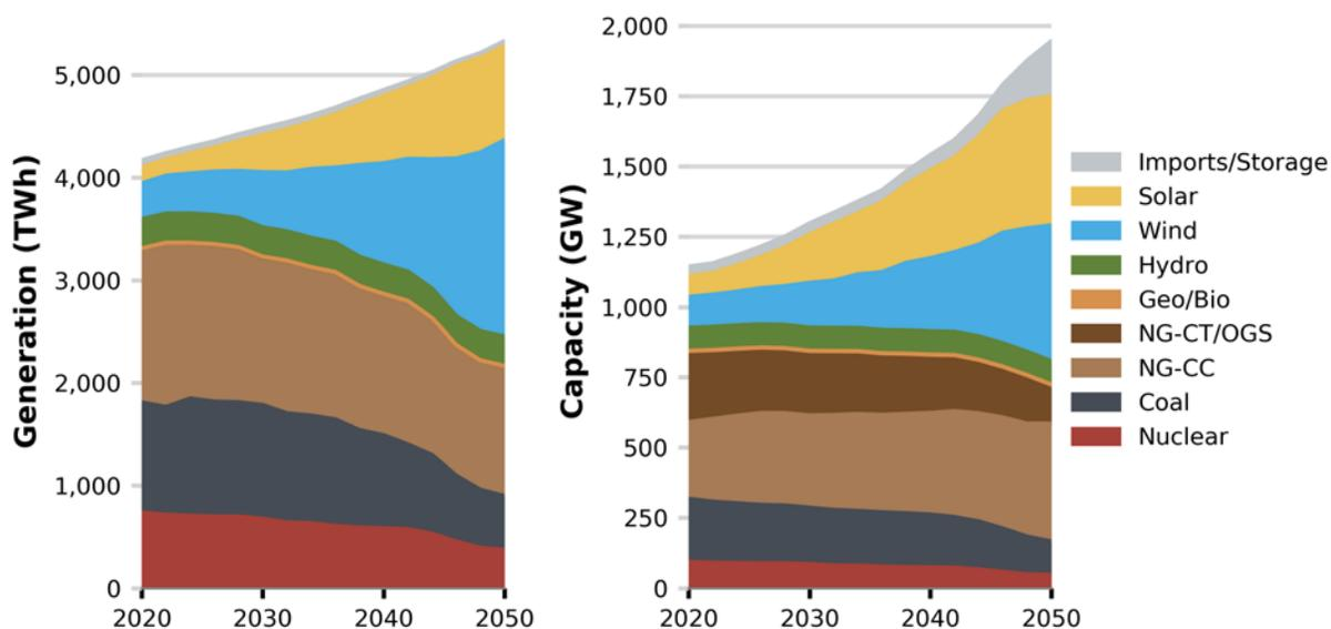
**Figure ES-1. U.S. power sector evolution over time for the Mid-case scenario.** The gray area represents imports from Canada in the left figure and storage capacity in the right figure. Storage generation is not shown because storage always has a negative net generation (due to losses). NG-CC is natural gas combined cycle, NG-CT is natural gas combustion turbine, OGS is oil-gas-steam, Geo/Bio is geothermal and biopower, TWh is terawatt-hours, and GW is gigawatts.
