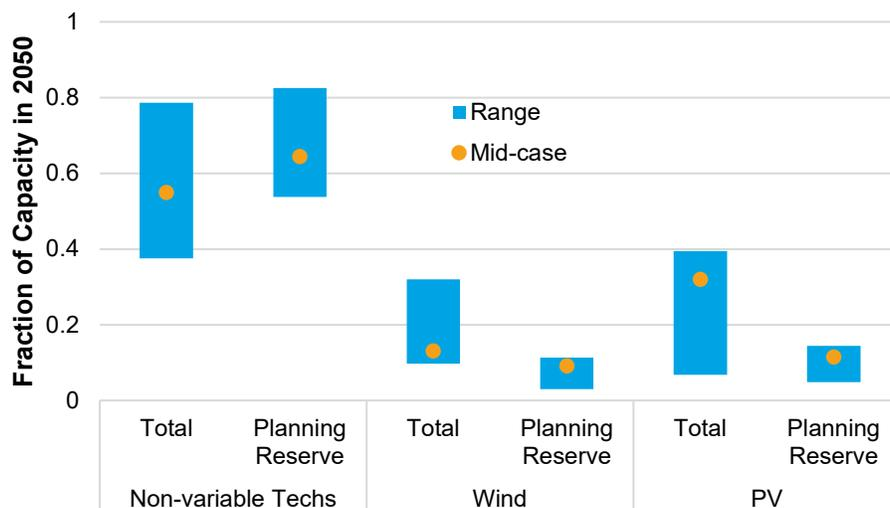
**Figure 15. Fraction of planning reserve contribution and total capacity from the specified technology types in 2050 in the summer.** The orange dots show the values from the Mid-case scenario, and the bars show the range across all the scenarios.
