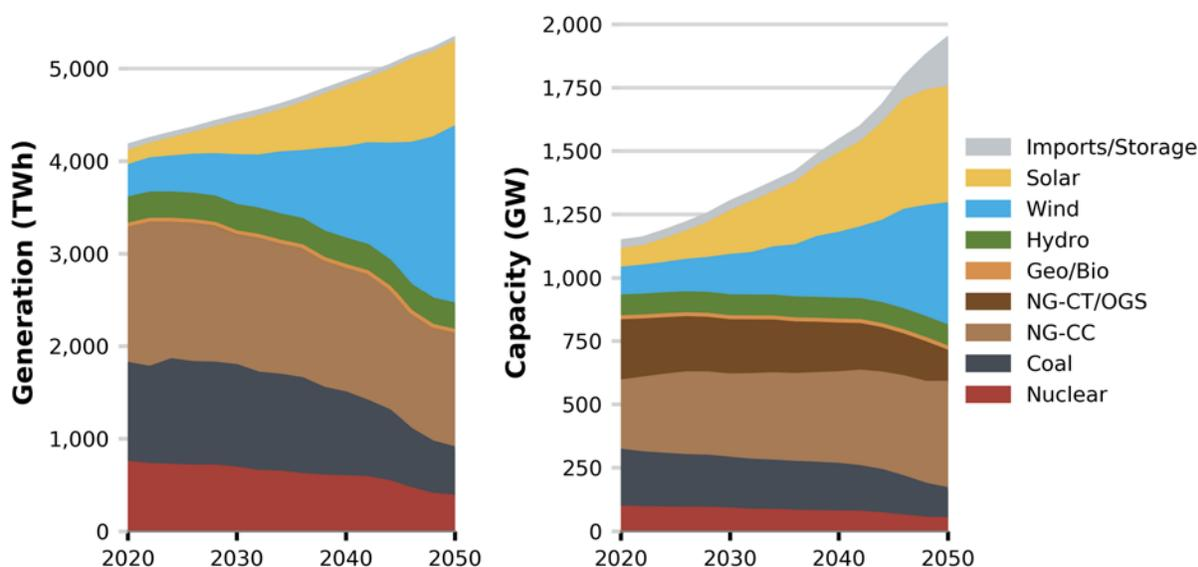
**Figure 2. U.S. power sector evolution over time for the Mid-case scenario.** The gray area represents imports from Canada in the left figure and storage capacity in the right figure. Storage generation is not shown because storage always has a negative net generation (due to losses). NG-CC is natural gas combined cycle, NG-CT is natural gas combustion turbine, OGS is oil-gas-steam, Geo/Bio is geothermal and biopower, and TWh is terawatt-hours.
