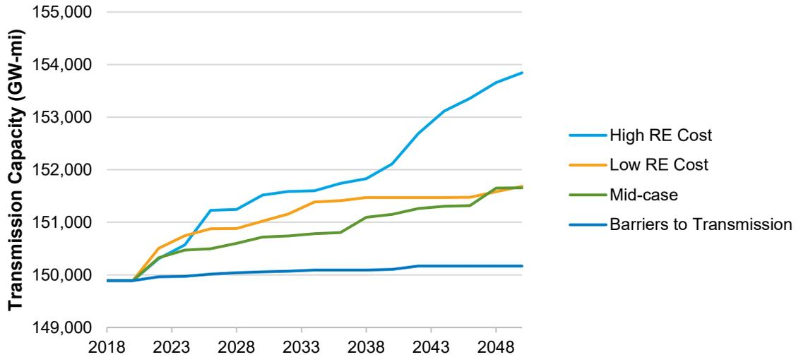
**Figure 22. National cumulative long-distance transmission capacity for the scenarios indicated.** This does not include the spur line transmission capacity used to connect RE resources into the bulk power system.
