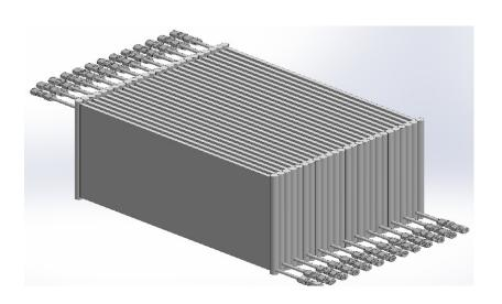
Can be improved to avoid multiple header welds, optimize solid side heat transfer and variable flow gaps, using combination of brazing and diffusion bonding of integral headers
