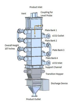
Shell-and-Plate Moving Packed Bed HX Design (Solex and VPE)
