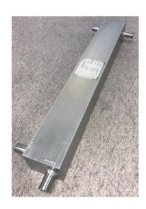
VPE provided compact heat exchangers for molten salt/CO2 application under IRP program.
