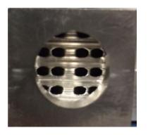
Flow channel size can be increased by facing typical PCHE channels each other – a cost effective approach than deep etching to create larger channel
