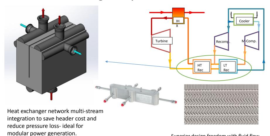
Cost is optimized using innovative channel layout that utilize pure multi-pass, counter flow.
