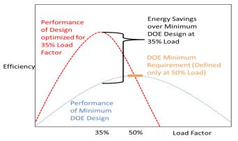
The EPA ENERGY STAR program recommends the following criteria for a meaningful level of energy savings above the DOE standard. Depending on load factor and output power, using these criteria *distribution transformer losses can be reduced by 11 to 29 percent*. (Throughout the remainder of the document, these criteria are referred to as "recommended energy efficiency criteria" and are implied when discussing "energy efficient transformer(s)".)
