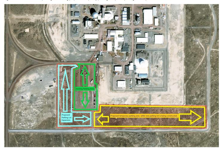
The gravel parking areas require road base from the Monroe gravel pit to bring them level with paved areas prior to paving the entire lot. Following paving, the proposed action adds bus drop-off and pick-up lanes to improve the safety of drivers and pedestrians and establishes a new drop off and entry adjacent to MFC-701.
