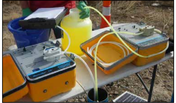
Left and right: Dr. Paul Reimus (LANL) oversees fluorescein dye tracer injection and pumping at the Grand Junction, Colorado, Site.
