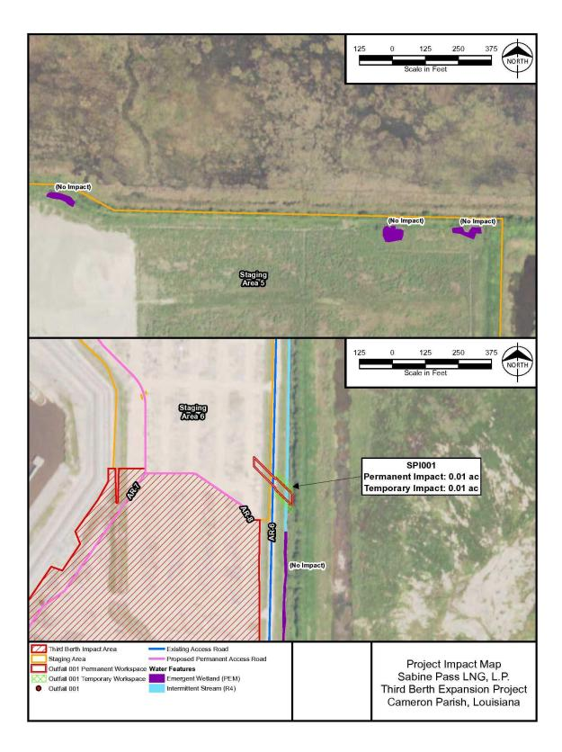
Figure B.3.2-2 Third Berth Expansion Project Wetland and Waterbody Impact Detail Map
