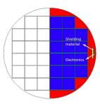
MNCP6 model to test the radiation shielding performance.
