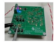
The electronics system PCB (partially populated) used to collect sensor signals and drive the through-wall communications.
