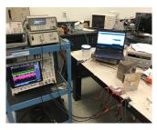
The experimental setup demonstrating data communication through steel enclosure material.
