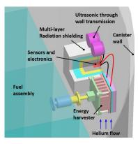
Energy harvester for powering sensing and communications.
