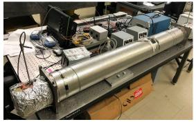
Figure 1. Laboratory setup for acoustic communication at elevated temperature using LiNbO<sub>3</sub> transducers
