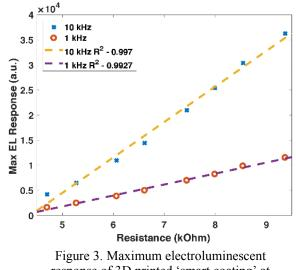
response of 3D printed 'smart coating' at various levels of resistance for two excitation features.
